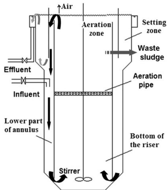
Fig. 1. Schematic structure of the ALR.
