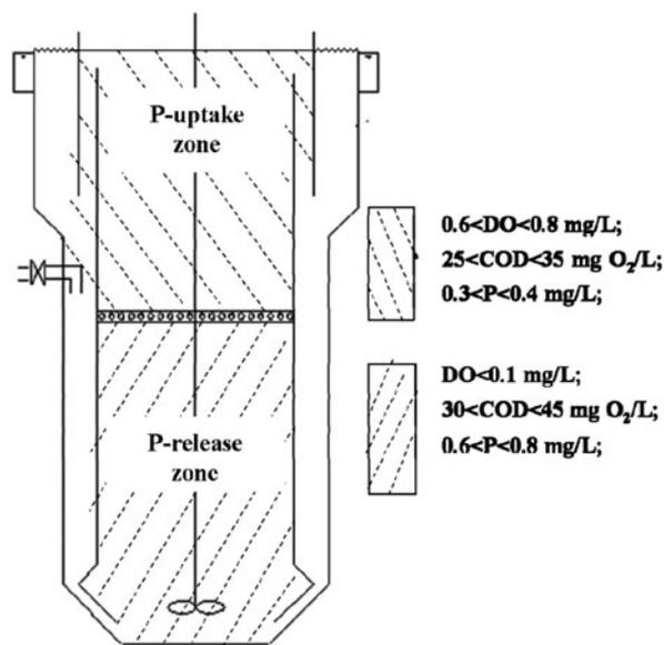
Fig. 5. P removal process in the ALR.
