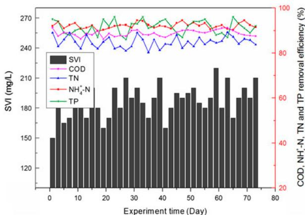
Fig. 2. Removal efficiency of TN, TP, COD, and  $\text{NH}_4^+-\text{N}$  under LFB state.
