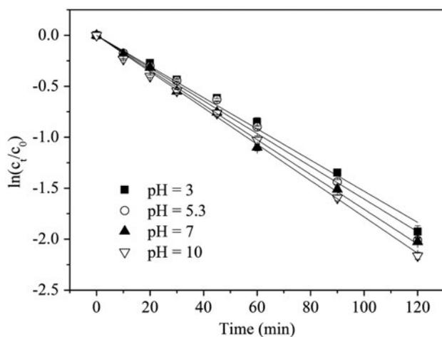
Fig. 3. Effect of initial pH on the degradation of SMX by heat-activated persulfate. ( $[\text{SMX}]_0 = 40 \mu\text{M}$ ,  $[\text{Na}_2\text{S}_2\text{O}_8]_0 = 2.4 \text{ mM}$ ,  $T = 60^\circ\text{C}$ .)
