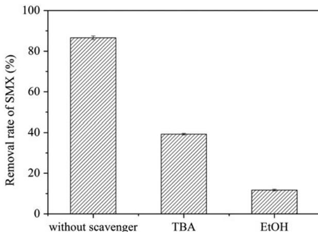
Fig. 5. SMX degradation without and with different scavengers. ( $[\text{SMX}]_0 = 40 \mu\text{M}$ ,  $[\text{Na}_2\text{S}_2\text{O}_8]_0 = 2.4 \text{ mM}$ ,  $[\text{TBA}]_0 = [\text{EtOH}]_0 = 0.96 \text{ M}$ ,  $T = 60^\circ\text{C}$ .)
