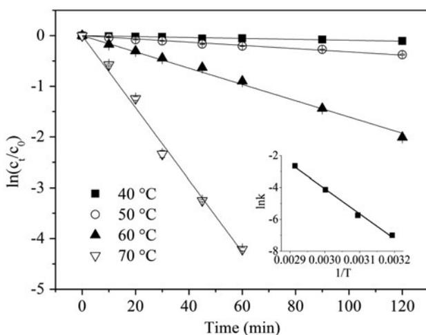
Fig. 1. Effect of temperature on the degradation of SMX by heat-activated persulfate. ( $[\text{SMX}]_0 = 40 \mu\text{M}$ ,  $[\text{Na}_2\text{S}_2\text{O}_8]_0 = 2.4 \text{ mM}$ ,  $T = 40, 50, 60, \text{ and } 70^\circ\text{C}$ ; insert: plot of  $\ln k$  vs.  $1/T$  for  $E_a$  estimation.)
