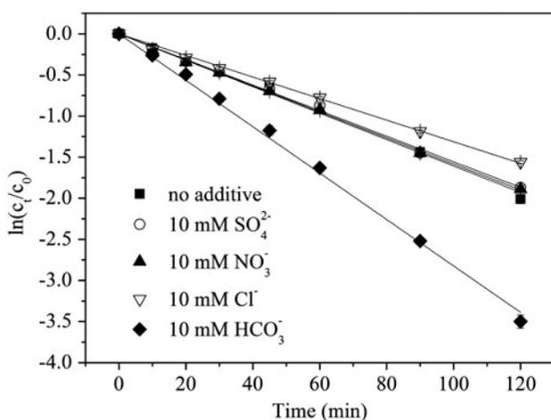
Fig. 4. Effect of anions on the degradation of SMX by the heat-activated persulfate process. ( $[\text{SMX}]_0 = 40 \mu\text{M}$ ,  $[\text{Na}_2\text{S}_2\text{O}_8]_0 = 2.4 \text{ mM}$ ,  $T = 60^\circ\text{C}$ ,  $[\text{Cl}^-]_0 = [\text{NO}_3^-]_0 = [\text{SO}_4^{2-}]_0 = [\text{HCO}_3^-]_0 = 10 \text{ mM}$ ).
