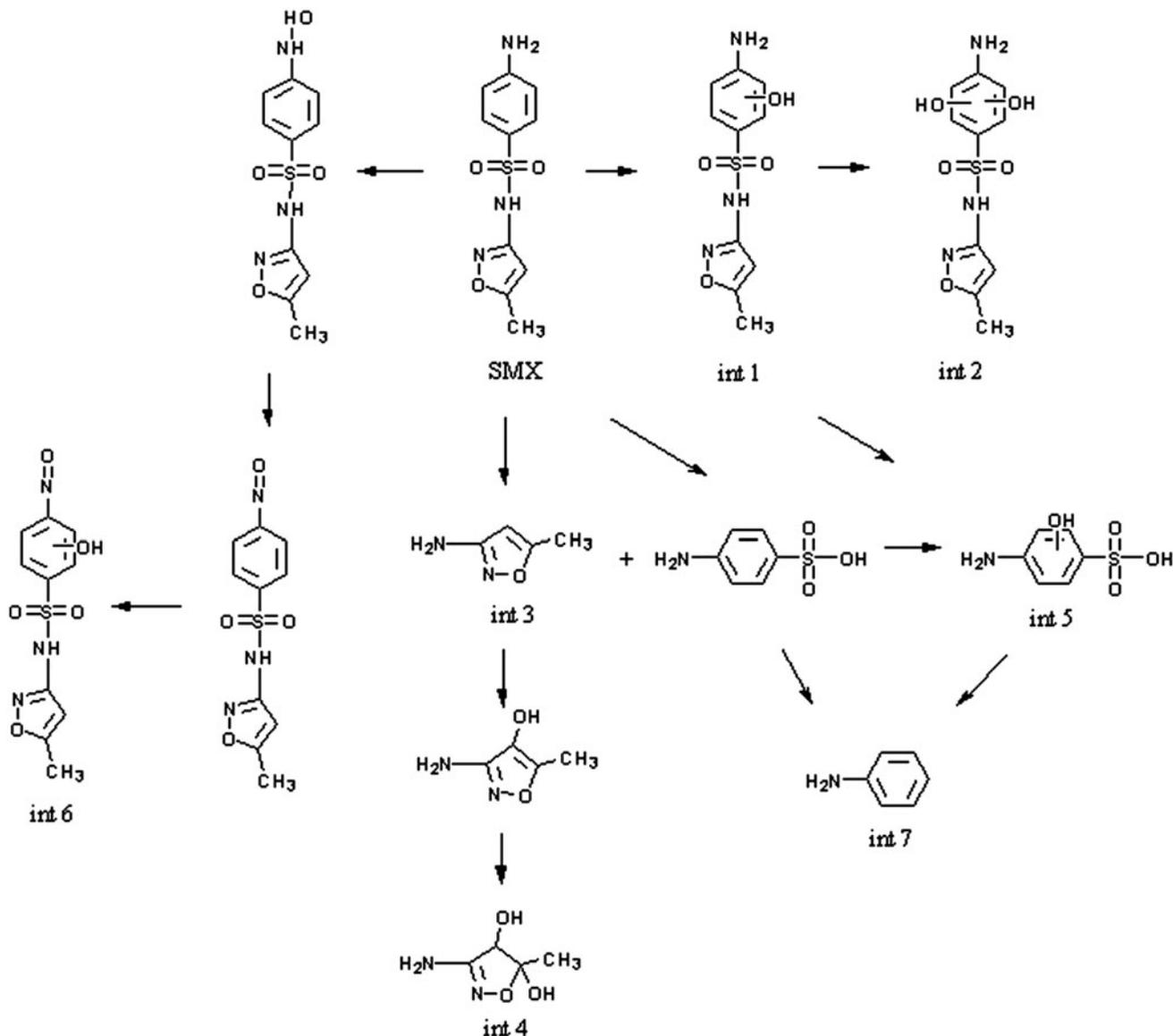
Fig. 6. Proposed reaction pathways for SMX degradation in the heat-activated persulfate system.
