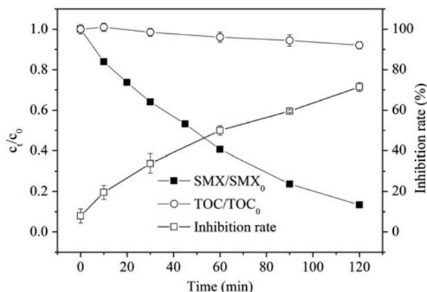
Fig. 7. Change of SMX/SMX<sub>0</sub>, TOC/TOC<sub>0</sub>, and toxicity during the oxidation process.
