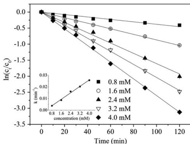
Fig. 2. Effect of persulfate dose on the degradation of SMX by heat-activated persulfate. ( $[\text{SMX}]_0 = 40 \mu\text{M}$ ,  $[\text{Na}_2\text{S}_2\text{O}_8]_0 = 0.8, 1.6, 2.4, 3.2$  and  $4.0 \text{ mM}$ ,  $T = 60^\circ\text{C}$ ; insert: plot of  $k$  vs.  $[\text{persulfate}]_0$ .)
