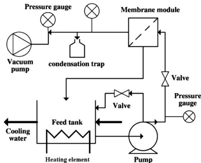
Fig. 2. Schematic diagram of VMD setup.
