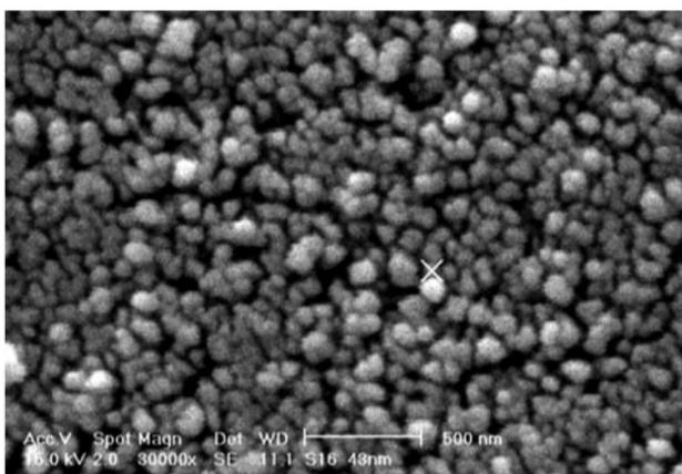
Fig. 2. The SEM micrograph of the ZnO nanoparticle.
