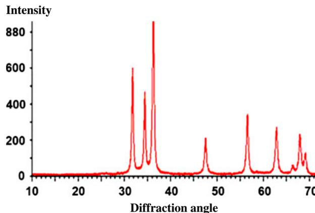
Fig. 1. XRD pattern of ZnO nanoparticle prepared with SCM.
