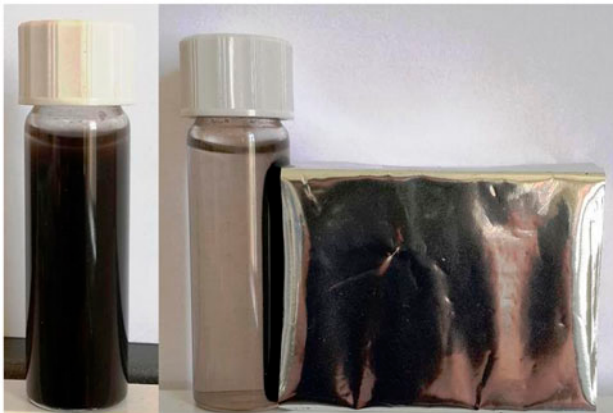
Fig. 3. Photograph of magnetic separation of AC-MIONs from solution.
