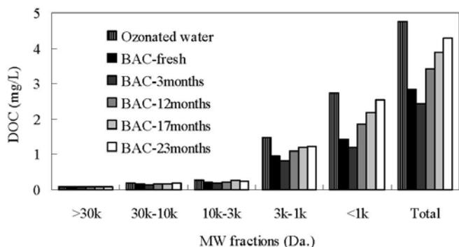
Fig. 6. DOC removal in different MW fractions for different BAC service periods.
