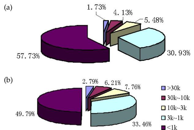
Fig. 5. MW distribution before (a) and after (b) BAC filtration.
