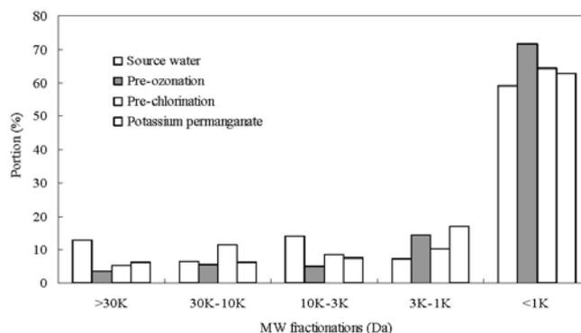
Fig. 3. MW distribution for source water by different pre-oxidation processes ( $\text{O}_3$  dosage: 1.2 mg/L;  $\text{Cl}_2$  dosage: 2.5 mg/L;  $\text{KMnO}_4$  dosage: 1.2 mg/L).
