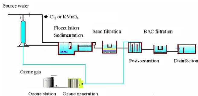
Fig. 2. Pilot-scale water treatment process.
