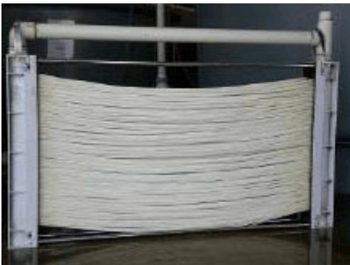
Fig. 2. Microfiltration membrane used in the MBR of the RAS.
