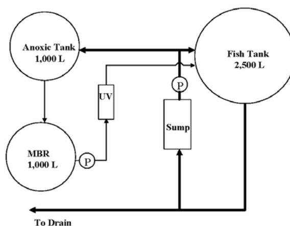
Fig. 1. Schematic of the RAS.
