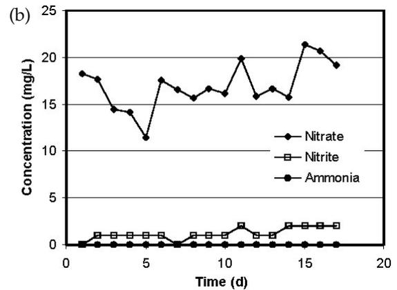
Fig. 6. Concentration of nitrogen species during the non-PAC run. (a) Fish tank. (b) Permeate from the MBR.
