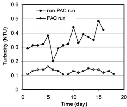
Fig. 5. Turbidity of the permeate from the MBR in both non-PAC and PAC runs.
