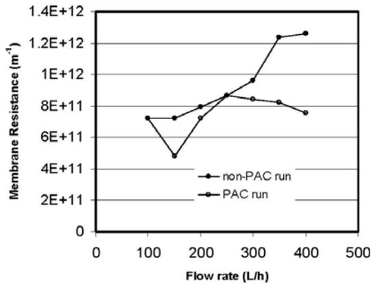
Fig. 4. Combined resistance due to membrane and irreversible fouling ( $R_m + R_f$ ) in both non-PAC and PAC runs.
