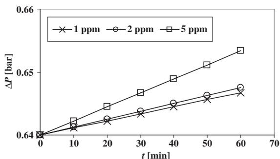
Fig. 7. TMP increase at  $J = 80 \text{ L/m}^2 \text{ h}$  for coagulant dose of 1, 2 and 5 mg  $\text{Al}^{3+}/\text{L}$ , at  $20^\circ\text{C}$ , total shear rate of 12,850, at ambient pH (7.4–7.7).
