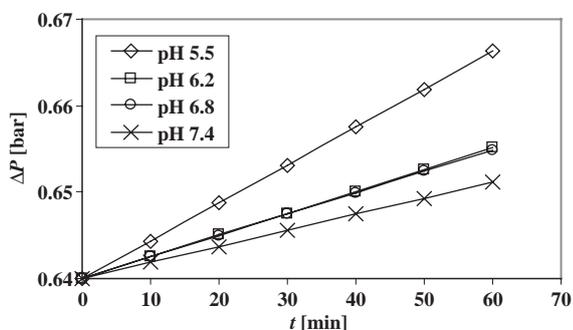
Fig. 8. TMP increase at  $J = 100 \text{ L/m}^2 \text{ h}$  for different pH values at coagulant dose of 5 mg  $\text{Al}^{3+}/\text{L}$ ,  $20^\circ\text{C}$  and no flocculation.
