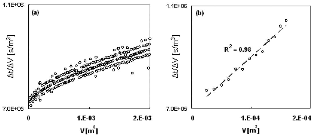
Fig. 9. Filtration curves for (a) tap water and (b) coagulated tap water at 5 mg Al<sup>3+</sup>/L, pH 6.8 and shear rate of 12,850.
