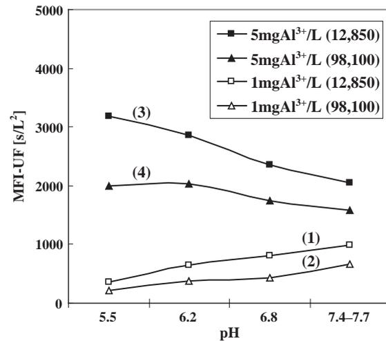
Fig. 4. Effect of increase in shear rate from 12,850 to 98,100 (1–35 min flocculation time) at different pH values for a coagulant dose of 1 and 5 mg Al<sup>3+</sup>/L.
