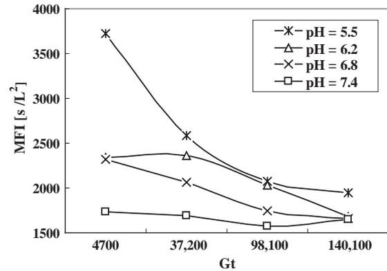
Fig. 5. Effect of pH and shear rate on MFI at 5 mg  $Al^{3+}/L$ .
