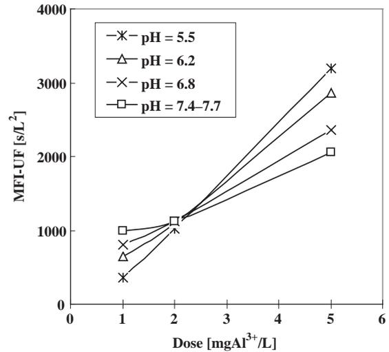
Fig. 2. MFI as a function of dose and pH at a constant shear rate of 12,850 (1 min flocculation time).
