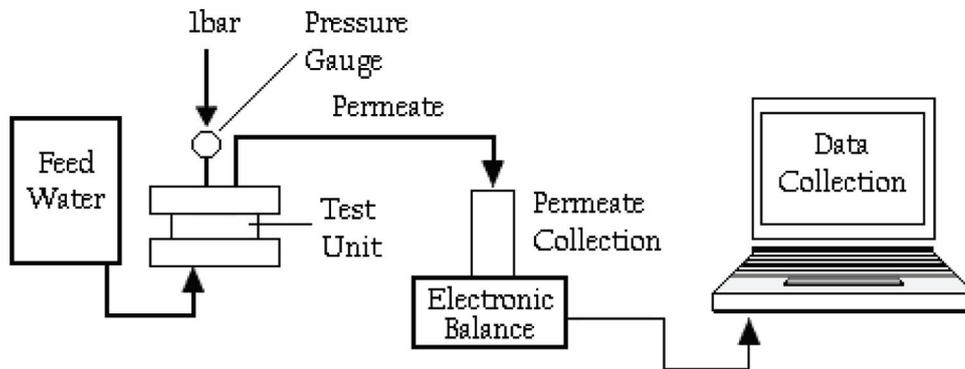
Fig. 1. Scheme of the filtration set-up.
