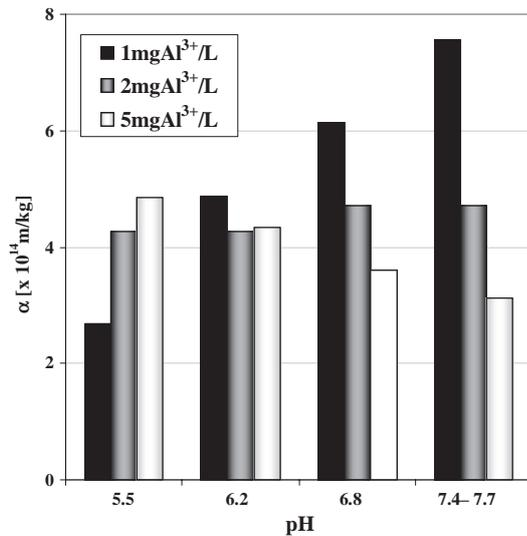
Fig. 3. Specific resistance of aluminium flocs at different dose and pH values at a total shear rate of 12,850 (1 min flocculation time).
