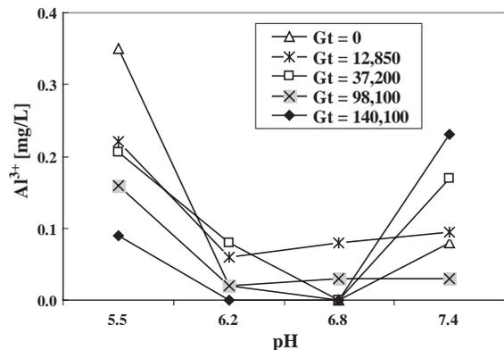
Fig. 6. Aluminium residual as a function of pH at coagulant dose of 5 mg  $Al^{3+}/L$  for different shear rates.
