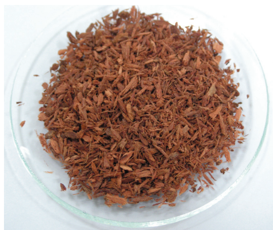
Fig. 2. Macroscopic structure of eucalyptus bark particle.
