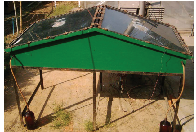
Fig. 1 (b). Photograph of double slope passive solar still.
