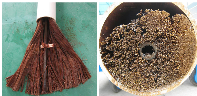
Fig. 18. Returned module from Wang Tan — autopsy before cleaning.
