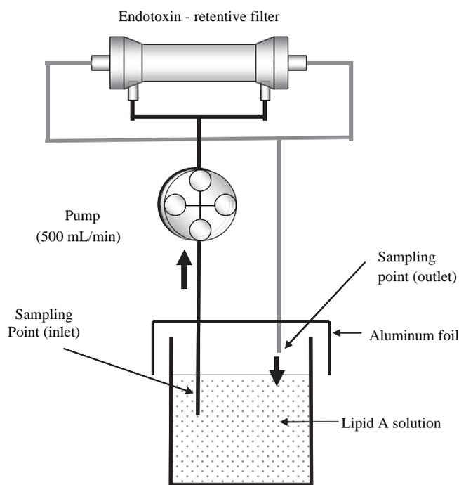
Fig. 1. Experimental apparatus for evaluation of the endotoxin-retentive filter. Filtration tests for lipid A were carried out by adding lipid A to the circulating water to concentrations ranging from 10 to 100 EU/L. The endotoxin-retentive filter was connected to a circulation circuit composed of silicone tubes. The lipid A solution was filtered from the shell-side to the lumen-side of the filter for 4 h at a flow rate of 30 L/h.
