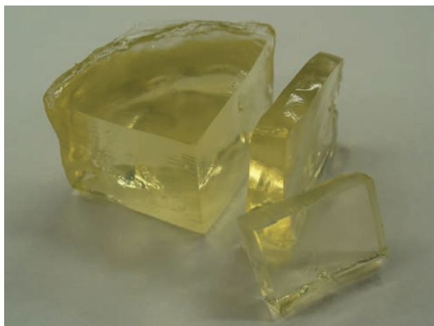
Fig. 2. The optical photograph of acetylated chitosan gel after 48 h which completed acetylation in Fig. 1.
