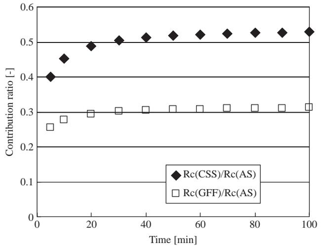
Fig. 4. Change of contribution ratio of filtration resistance with time.
