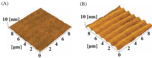
Fig. 1. AFM images of polyimide surfaces: (A) Unrubbed surface and (B) rubbed surface.
