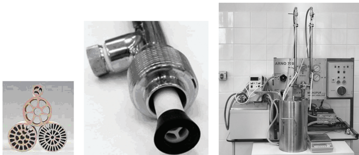
Fig. 2. ARNO 700 lab-scale filtration unit with three channel membrane type Clover.
