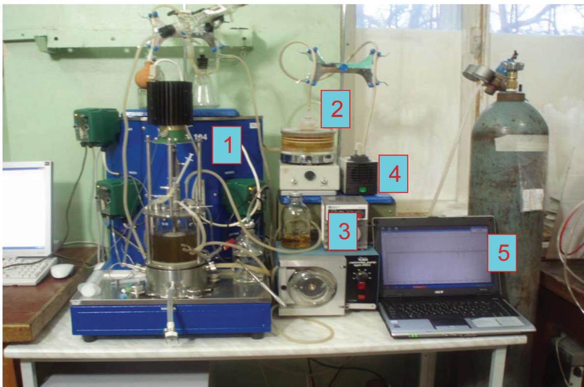
Fig. 5. Laboratory set of equipment for continuous thermophilic cellulose fermentation integrated with membrane module. 1 – anaerobic reactor, 2 – membrane module, 3 – peristaltic pump, 4 – vacuum pump, 5 – PC with program control of overall fermentation process.
