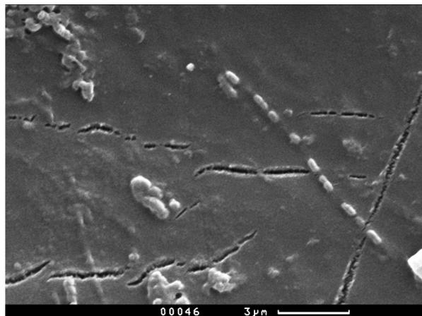
Fig. 2. Electronic microphotography of PVTMS membrane surface after 4 weeks of incubation in the medium with active microbial consortia, degrading cellulose.
