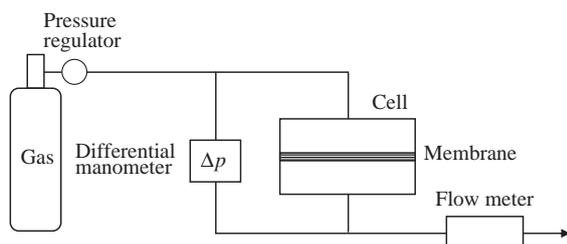
Fig. 1. The scheme of the setup for membrane permeance measurement.
