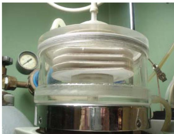
Fig. 4. The frontal view of membrane module mounted into plastic container.
