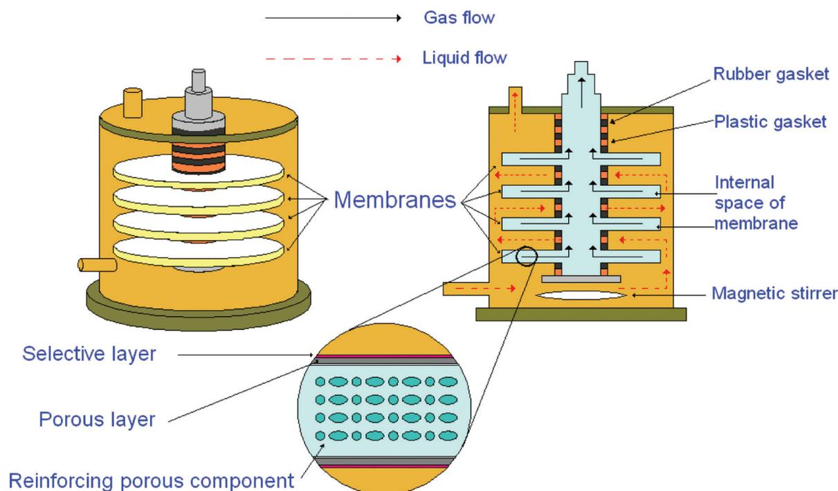
Fig. 3. Membrane module construction.
