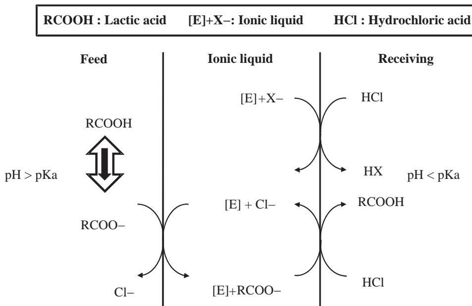
Fig. 10. Permeation mechanism of lactic acids with supported ionic liquid membrane.
