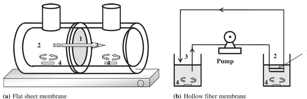
Fig. 1. Experimental apparatus: (1) supported ionic liquid membrane; (2) feed solution; (3) stripping solution; (4) stirring bar.
