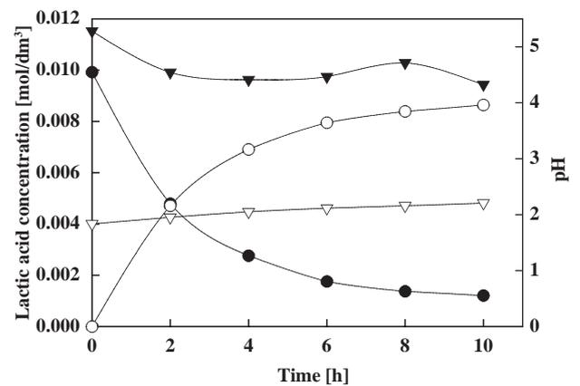
Fig. 15. Time courses of lactic acid concentration in feed (●) and stripping (○), and pH of feed (▼) and stripping (▽) phases using Aliquat 336 impregnated hollow fiber membranes, 0.01 mol/dm<sup>3</sup> lactic acid and 0.02 mol/dm<sup>3</sup> hydrochloric acid as membrane, feed and stripping solutions, respectively.
