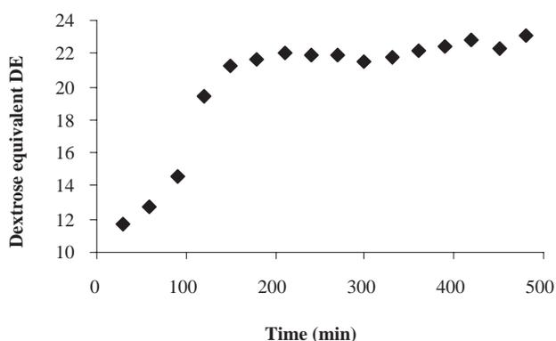
Fig. 3. Time dependence of DE of components in permeate during enzymatic hydrolysis of P 0.5% Ac starch (15 and 50 kDa membranes).
