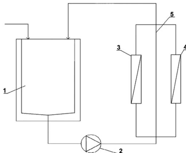
Fig. 1. Schematic diagram of system studied. 1 – reaction vessel; 2 – rotary lobe pump; 3, 4 – ultrafiltration module; 5 – bypass.
