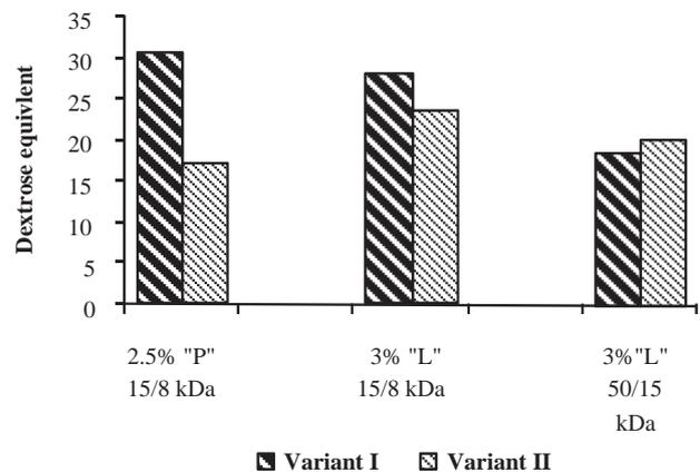
Fig. 8. Dextrose equivalent of hydrolysis products after 150 min of process.
