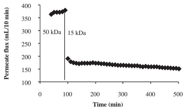
Fig. 4. Time dependence of permeate flux for hydrolysis on membrane module 50/15 kDa.
