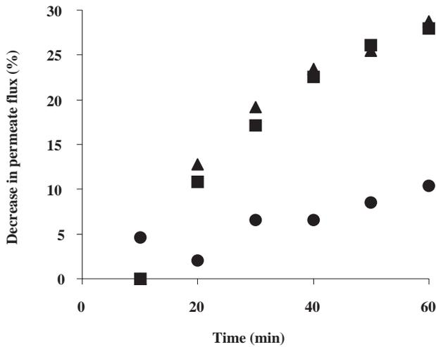
Fig. 5. Change of permeate flux of pudding 2.5% Ac modified starch during first 60 min of separation process for 15 kDa membrane: 15 kDa (▲), 15/8 kDa (■), 50/15 kDa (●).
