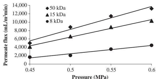
Fig. 2. Dependence of pure water flux on transmembrane pressure for membranes with cut off 8, 15 and 50 kDa.
