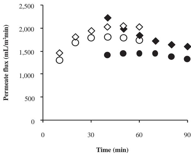
Fig. 6. Time dependence of permeate flux for hydrolysis on first module (15 kDa membrane). Variant I: ▲ 2.5% P, ● 3% L, Variant II: △ 2.5% P, ○ 3% L.
