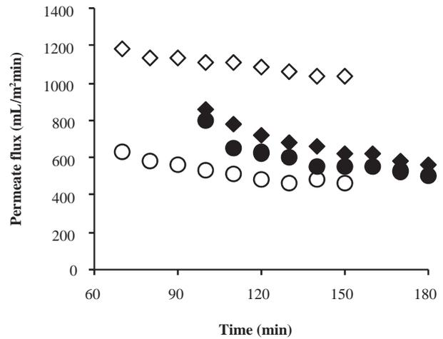
Fig. 7. Time dependence of permeate flux for hydrolysis on second module (8 kDa membrane). Variant I: ▲ 2.5% P, ● 3% L, Variant II: △ 2.5% P, ○ 3% L.
