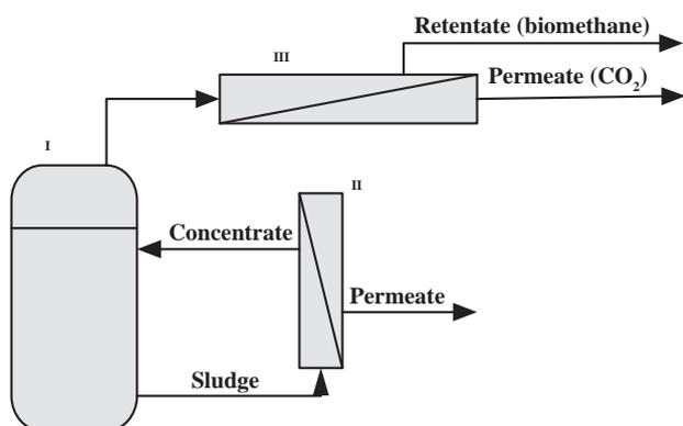
Fig. 1. Schematic representation of the anaerobic membrane bioreactor: I anaerobic fermenter, II membrane filtration unit, III gas separation unit.
