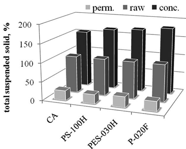
Fig. 4. TSS results for the examined UF membranes.
