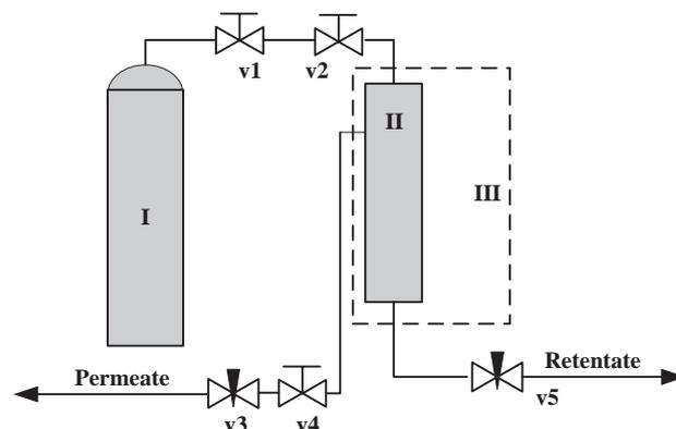
Fig. 2. Flowsheet of GC-MS 100 high pressure gas-separation unit: I gas-cylinder, II membrane module, III thermostat.
