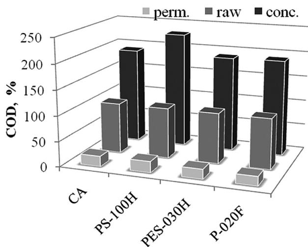
Fig. 3. COD results for the examined UF membranes.
