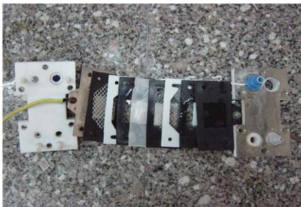
Fig. 4. Side view of the membrane cell used in this study, Cell body (Teflon), EPDM gasket, Standard DSA/Cl<sub>2</sub> anode, Flemion 892 membrane, Nickel cathode, Flow frame (Teflon), Electrolyte inlet, Electrolyte outlet.
