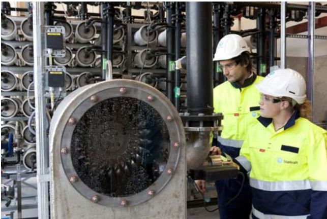
Fig. 7. The turbine generating electricity in the osmotic power prototype.
