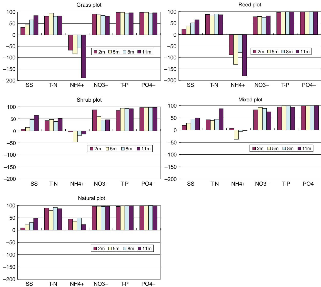
Fig. 7. Removal effectiveness of pollutants by width of each plot. X-axis corresponds to pollutants, while the Y-axis corresponds to removal efficiency (%).
