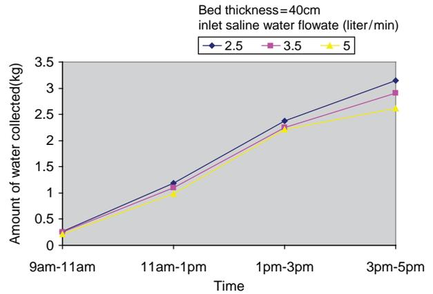
Fig. 16. Amount of pure water collected versus time for different inlet saline water flow rates without exit brine recycling.
