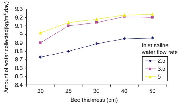
Fig. 15. Amount of water collected versus bed thickness for different inlet saline water flow rates.
