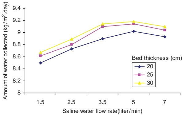
Fig. 13. Amount of water collected versus inlet saline water flow rate for different bed thickness.
