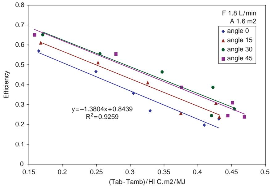
Fig. 3. Efficiency of the solar collector at different angles of inclination.
