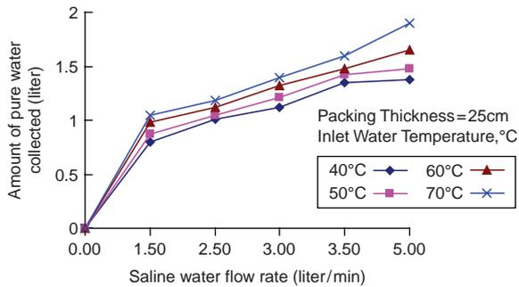
Fig. 9. Amount of pure water collected versus saline water flow rate for different inlet water temperatures.
