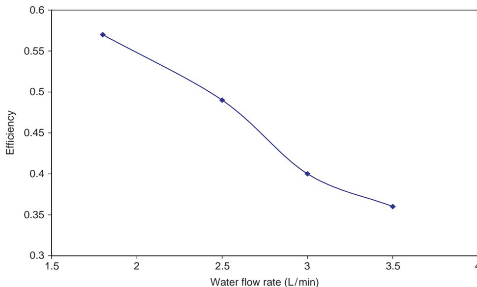
Fig. 8. Effect of changing the water flow rate on the efficiency of the solar collector in the HD unit.
