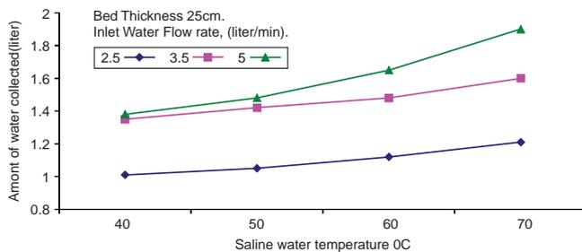
Fig. 10. Amount of water collected versus saline water inlet temperature at different inlet water flow rates.
