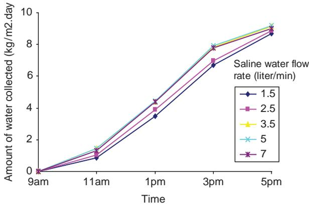
Fig. 12. Amount of water collected distributed from 9 am up to 5 pm for different inlet saline water flow rates.
