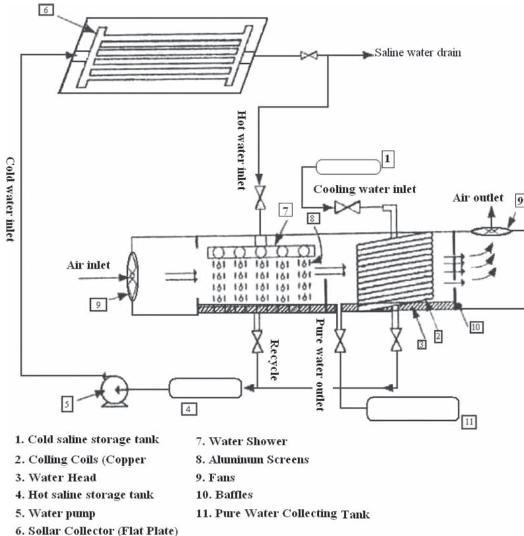
Fig. 1. Schematic diagram of saline water desalination system by humidification dehumidification process using solar energy.
