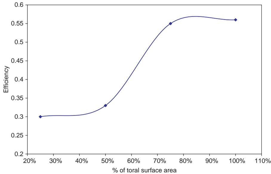
Fig. 6. Effect of changing the area of the solar collector on its efficiency.
