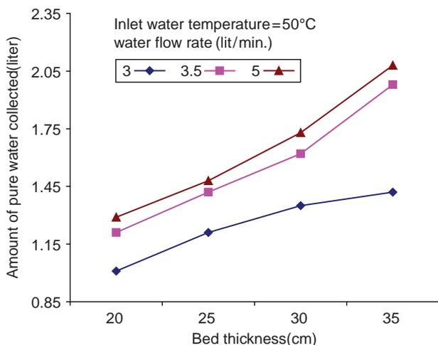
Fig. 11. Amount of pure water collected versus Bed thickness at different inlet water flow rates.
