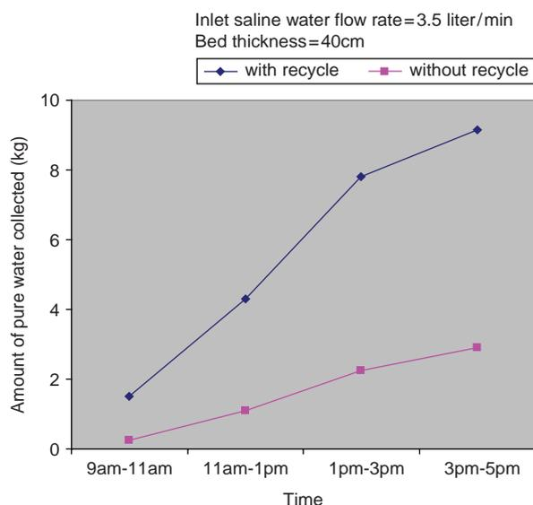
Fig. 17. Amount of pure water collected versus time with and without exit brine recycling
