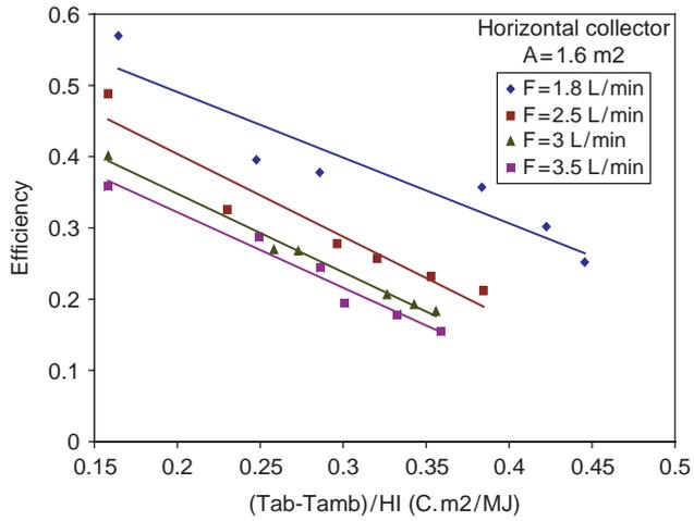
Fig. 7. Efficiency of the solar collector at different saline water flow rates.
