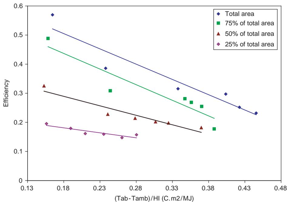
Fig. 5. Efficiency of the solar collector at different surface area of the collector.
