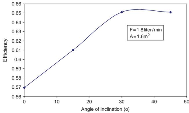
Fig. 4. Effect of changing the angle of inclination on the efficiency of the solar collector.
