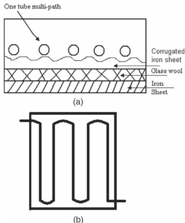
Fig. 2. Details of the solar collector used in the desalination units: (a) sketch of flat plate solar collector; (b) sketch of the pathway in the solar collector.
