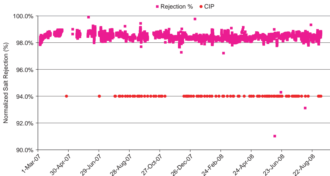
Fig. 6. Normalized Salt Rejection of skid 1.
