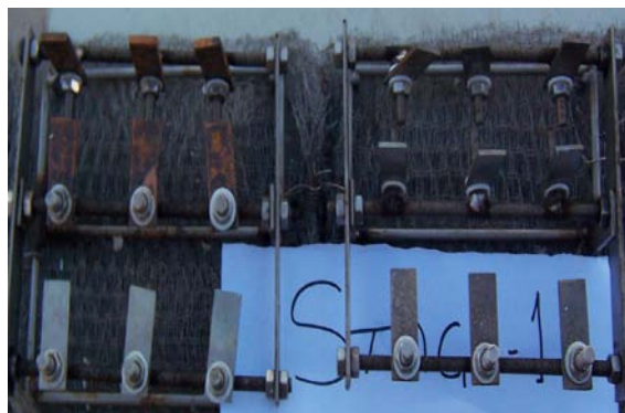
Fig. 7. The photograph shows the appearance of coupons after the test completion at 100°C (TBT) at stage one.
