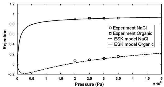
Fig. 5. Solute rejection of binary solutes system plotted against pressure using the experimental data and simulation results from the extended Spiegler–Kedem model by incorporating osmotic coefficient (new method).
