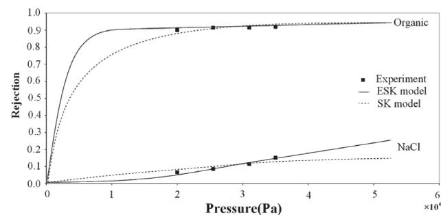
Fig. 2. Solute rejection of binary solutes system plotted against pressure using the experimental data and simulation results from the extended Spiegler–Kedem model [7].
