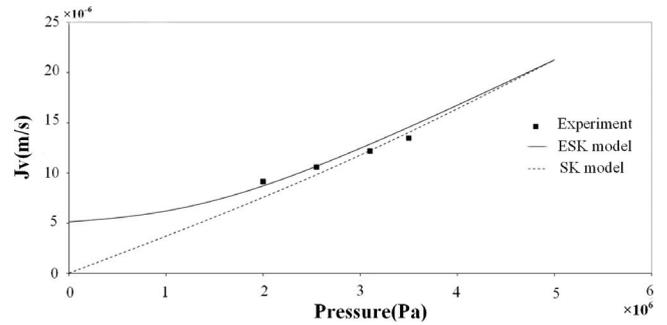
Fig. 3. Volumetric flux of binary solutes system of NaCl and organic matters of sugarcane plotted against pressure using the experimental data [13] and simulation results from the extended Spiegler–Kedem model [7].
