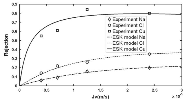
Fig. 8. Ions rejection of  $\text{CuCl}_2$ , NaCl system versus volumetric flux from the simulation results of the extended Spiegler–Kedem model (new method).
