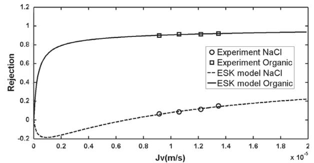
Fig. 4. Solute rejection of binary solutes system plotted against volumetric flux from the simulation results of the extended Spiegler–Kedem model (new method).
