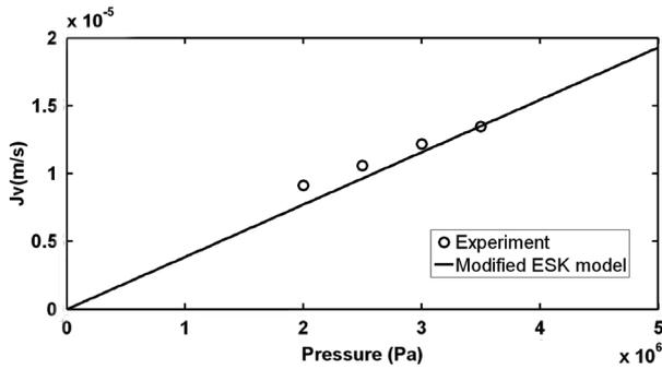
Fig. 6. Volumetric flux of binary solutes system of NaCl and organic matters of sugarcane plotted against pressure using the experimental data [13] and simulation results from the extended Spiegler–Kedem model by incorporating osmotic coefficient (new method).
