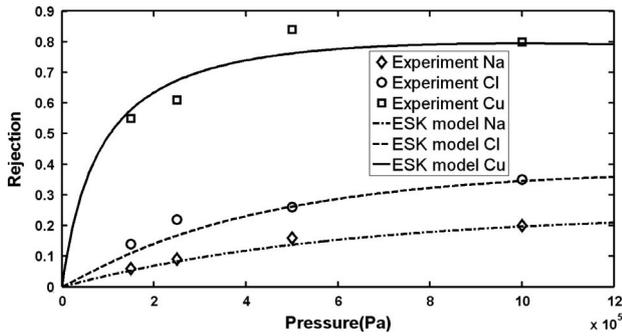
Fig. 10. Solute rejection of CuCl<sub>2</sub>, NaCl system plotted against pressure using the experimental data and simulation results from the extended Spiegler–Kedem model (new method).
