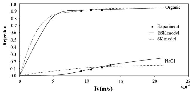
Fig. 1. Solute rejection of binary solutes system plotted against volumetric flux using the experimental data and simulation results from the extended Spiegler–Kedem model [7].
