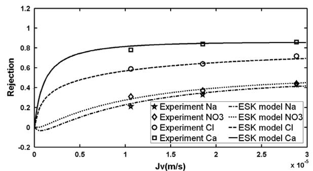
Fig. 12. Ions rejection of NaNO<sub>3</sub>/NaCl/CaCl<sub>2</sub> system versus volumetric flux. Experimental data and extended Spiegler–Kedem model using GA method simulations.
