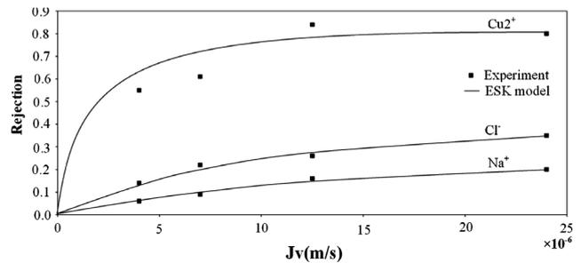
Fig. 7. Ions rejection of  $\text{CuCl}_2$ , NaCl system versus volumetric flux from the simulation results of the extended Spiegler–Kedem model [7].
