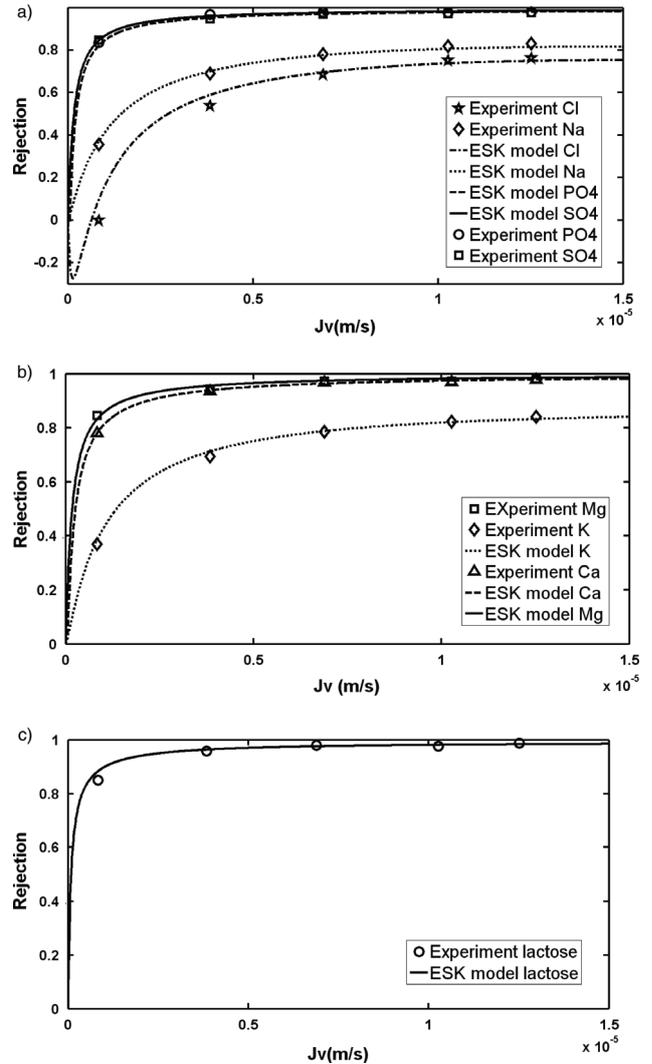
Fig. 13. Ions rejection of UF-whey system versus volumetric flux. Experimental results and extended Spiegler-Kedem model by using GA method simulations. (a) Cl<sup>-</sup>, Na<sup>+</sup>, PO<sub>4</sub><sup>3-</sup>, SO<sub>4</sub><sup>2-</sup>; (b) Mg<sup>2+</sup>, K<sup>+</sup>, Ca<sup>2+</sup>; (c) lactose.
