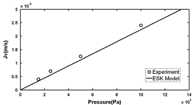
Fig. 9. Volumetric flux of  $\text{CuCl}_2$ , NaCl system plotted against pressure using the experimental data (circles) and simulation results from the extended Spiegler–Kedem new model (line).
