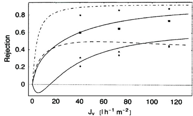
Fig. 11. Ions rejection of NaNO<sub>3</sub>/NaCl/CaCl<sub>2</sub> system versus volumetric flux. Experimental data and Nanoflux simulations [21]. Nanoflux predictions (data): dot-dashed curve (stars), Ca<sup>2+</sup>; upper solid curve (squares), Cl<sup>-</sup>; dashed curve (triangles), NO<sub>3</sub><sup>-</sup>; lower solid curve (diamonds), Na<sup>+</sup>.
