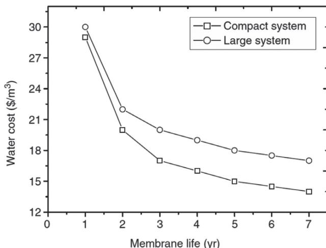
Fig. 14. The effect of increasing the plant lifetime on the distilled water cost [81].
