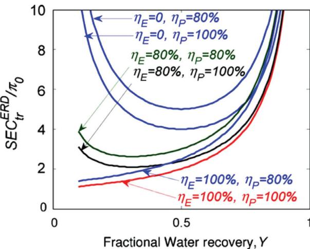
Fig. 5. Normalized SEC with ERD for single-stage RO system with pump efficiency,  $\eta_p$  and ERD efficiency,  $\eta_E$  at salt rejection of 99% [34].
