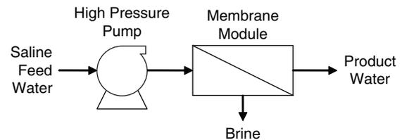
Fig. 2. Single-stage module arrangement [33].
