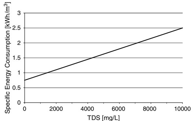
Fig. 13. Energy consumption of the RO desalination sub-unit as a function of TDS [53].
