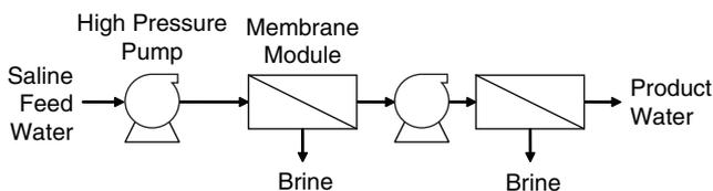
Fig. 7. Two-pass RO system without an ERD.
