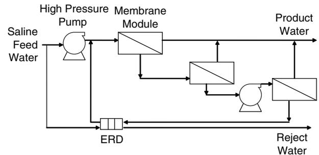
Fig. 11. Optimum module arrangement for feed concentration of 6000 mg/l [43].
