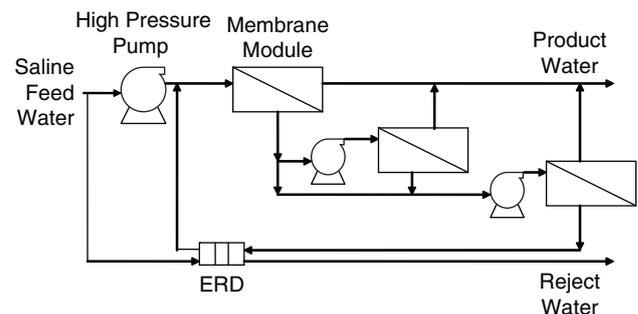
Fig. 12. Optimum module arrangement for feed concentration of 12,000 mg/l [43].
