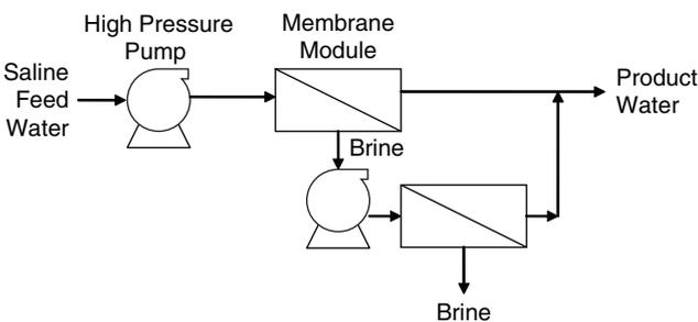
Fig. 6. Single-stage module arrangement with module connected to reject water with booster pump [33].
