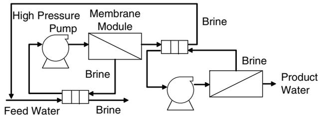
Fig. 9. Two-pass with ERD and recycling the concentrate of the second-pass to the feed water of the first-pass.
