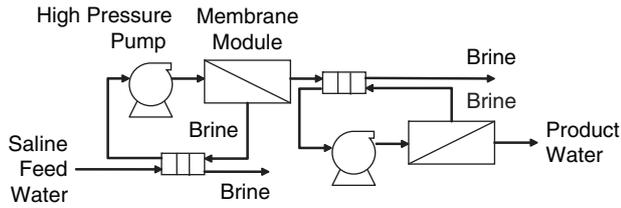
Fig. 8. Two-pass with ERD.
