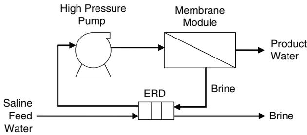
Fig. 4. Single-stage module arrangement ERD.
