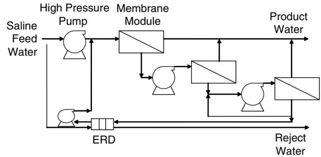
Fig. 10. Optimum module arrangement for feed concentration of 3000 mg/l [43].
