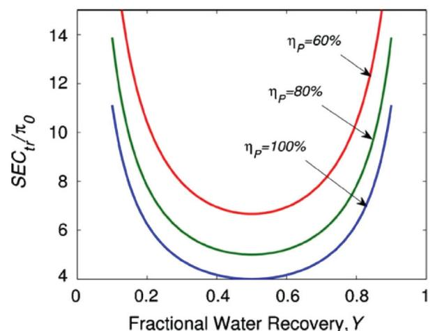
Fig. 3. Normalized SEC for single-stage RO system with pump efficiency,  $\eta_p$ , at salt rejection of 99% [34].
