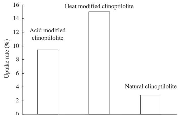
Fig. 3. Compared uptake rates (%) for methylene blue removal on natural, acid and heat modified treatment of clinoptilolite at 303 K and pH 7.0.
