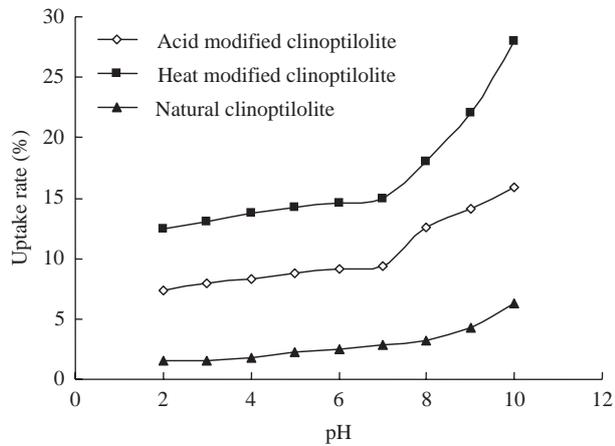
Fig. 2. Effect of pH on methylene blue adsorption on acid and heat treatment of clinoptilolite at 303 K.
