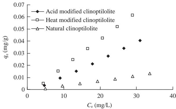
Fig. 4. The adsorption isotherms of methylene blue using the natural, acid and heat modified treatment of clinoptilolite at 303 K and pH 7.0
