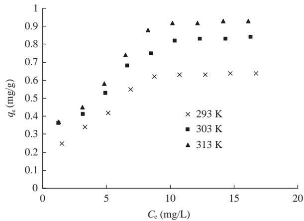
Fig. 5. Adsorption isotherms of methylene blue on the heat modified clinoptilolite at different temperatures.
