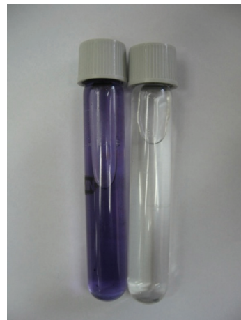
Fig. 1. Untreated textile dyehouse wastewater sample and reactor effluent after SCWO (550 °C).
