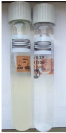
Fig. 6. Untreated cheese whey sample (left) and the 550°C reactor effluent sample after SCWO.
