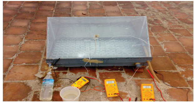
Fig. 2. Photograph of the honeycomb double exposure solar still.
