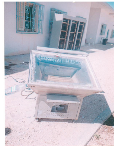
Fig. 2. Hybrid simple solar distiller/heat pump still: a) Schematic diagram of the still, b) Photograph of the SSDHP still.
