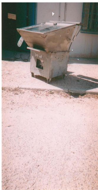
Fig. 1. Simple solar distiller still: a) Schematic diagram of the still, b) Photograph of the SSD still.
