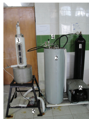
Fig. 1. Experimental setup of CO 2 hydrate formation (1) CO 2 storage tank, (2) ice water batch, (3) hydrate reactor, (4) CO 2 intermediate storage tank, (5) ice water pump, (6) refrigeration system.
