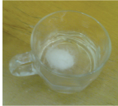
Fig. 2. Decomposing CO 2 hydrate crystal.
