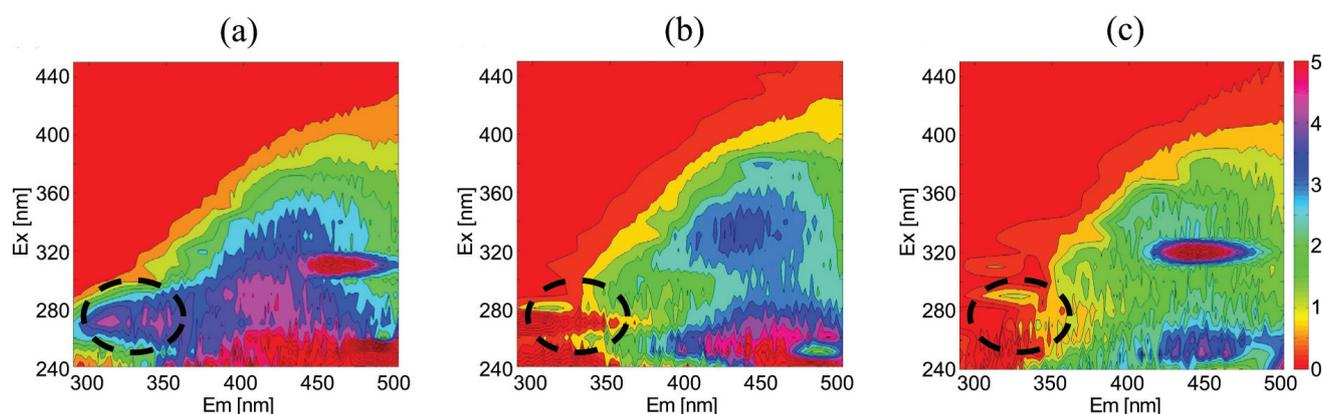
Fig. 6. Differential EEMs of the ultrafiltration tests using (a) secondary effluent, (b) SSF filtrate, (c) UF permeate of SSF filtrate (each based on samples taken after 1 h of filtration).
