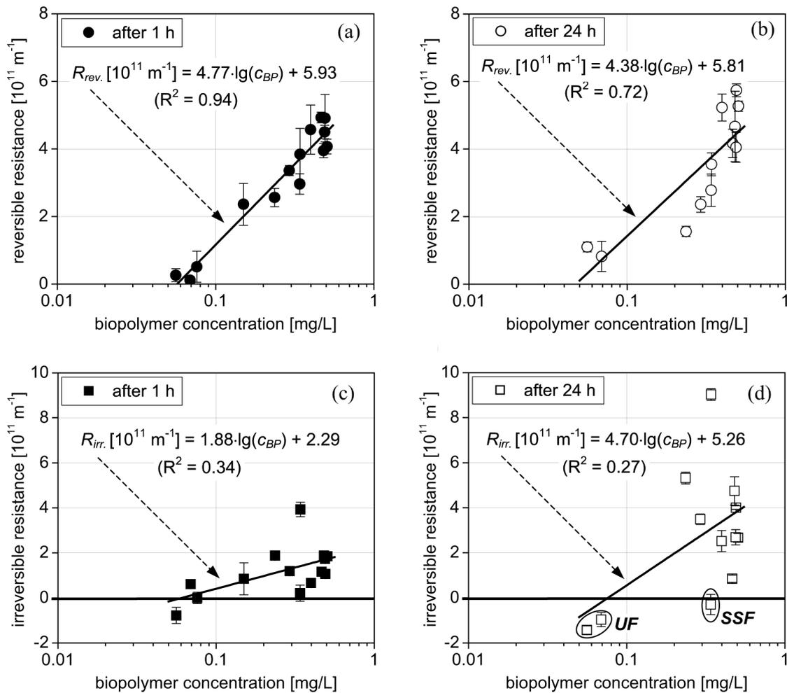
Fig. 4. Correlation between the biopolymer concentration  $c_{BP}$  (as carbon concentration) of different effluents and (a) hydraulically reversible resistance after 1 h, (b) hydraulically reversible resistance after 24 h, (c) hydraulically irreversible resistance after 1 h, (d) hydraulically irreversible resistance after 24 h.
