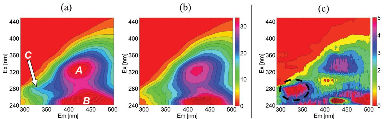
Fig. 5. EEMs of the ultrafiltration test using supernatant of MBR sludge after 1 h of filtration — (a) feed, (b) permeate, (c) differential EEM: (a)–(b).
