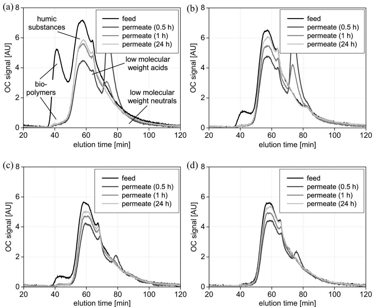
Fig. 2. LC–OCD chromatograms of feed and permeate samples of the ultrafiltration tests using (a) supernatant of MBR sludge, (b) secondary effluent, (c) SSF filtrate, (d) UF permeate of SSF filtrate (each sample threefold diluted; peaks at  $t \approx 75$  min are due to solvent residues originating from the membranes).
