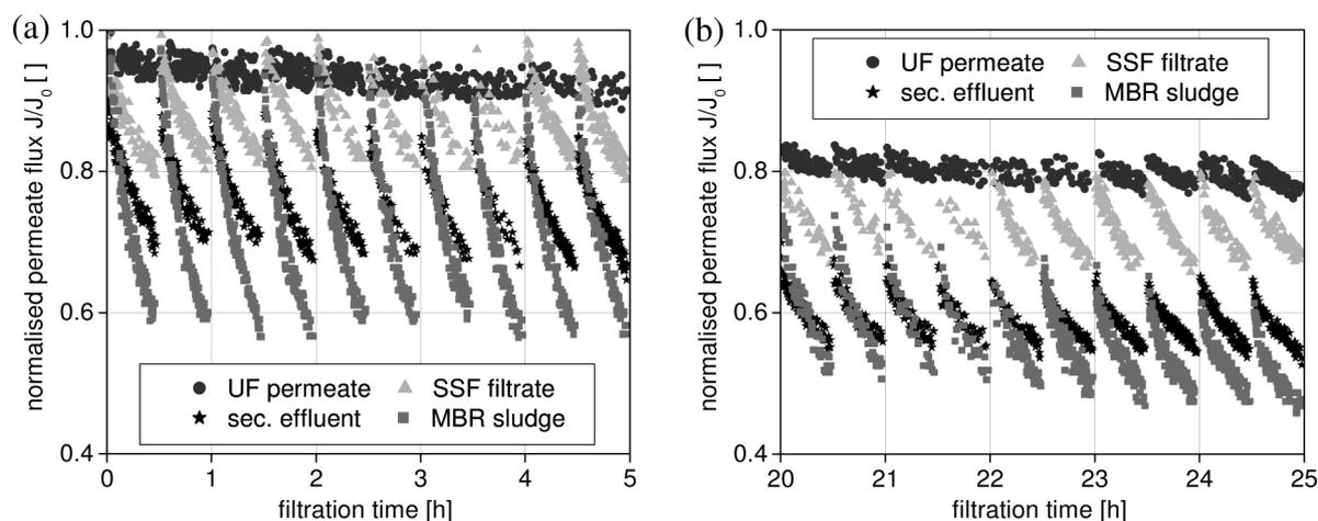
Fig. 1. Normalised permeate flux of ultrafiltration tests using supernatant of MBR sludge (DOC = 13.1 mg·L<sup>-1</sup>), secondary effluent (DOC = 10.9 mg·L<sup>-1</sup>), slow sand filter (SSF) filtrate (DOC = 9.4 mg·L<sup>-1</sup>), and SSF filtrate’s UF permeate (DOC = 8.7 mg·L<sup>-1</sup>) (a) in the initial phase, (b) at the end of the tests ( $J_0$ : initial permeate flux).
