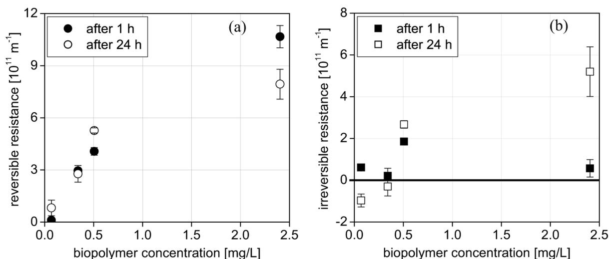
Fig. 3. Filtration resistances vs. biopolymer concentration (as carbon) of the ultrafiltration tests using supernatant of MBR sludge, secondary effluent, SSF filtrate, and UF permeate of SSF filtrate — (a) hydraulically reversible resistance, (b) hydraulically irreversible resistance (negative resistances are due to permeate fluxes after backwashing being slightly higher than in ultrafiltration of ultrapure water).
