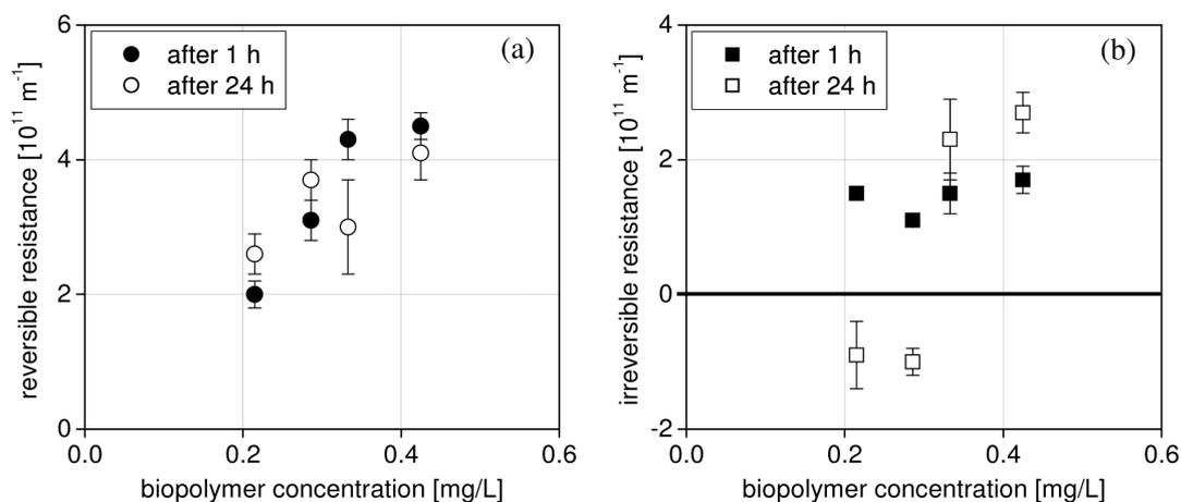
Fig. 8. Filtration resistances vs. biopolymer concentration (as carbon) of the ultrafiltration tests using untreated secondary effluent with and without previous coagulation – (a) hydraulically reversible resistance, (b) hydraulically irreversible resistance.
