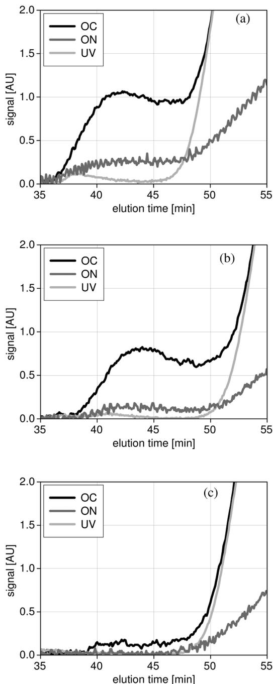
Fig. 7. Organic carbon (OC), organic nitrogen (ON) and  $UV_{254\text{ nm}}$  (UV) signals of the LC–OCD biopolymer fraction – (a) secondary effluent, (b) SSF filtrate, (c) UF permeate of SSF filtrate (each sample threefold diluted).
