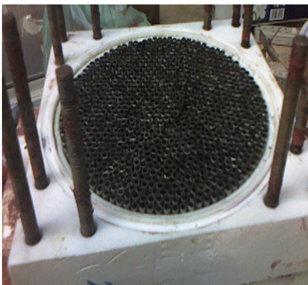
Fig. 2. The tubes bundle electrode (6 mm diameter tubes).
