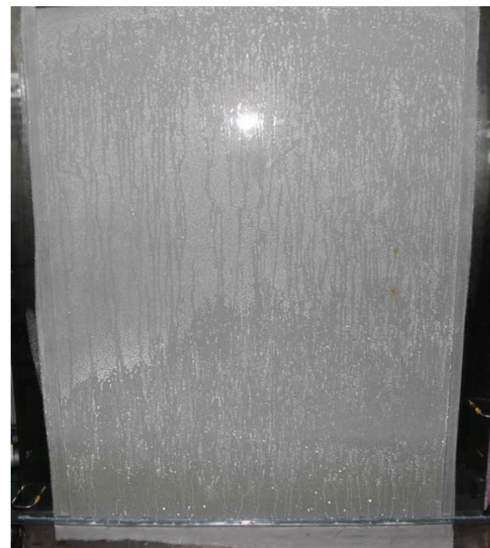
Fig. 8. Distilled water on the condensing glass plate.
