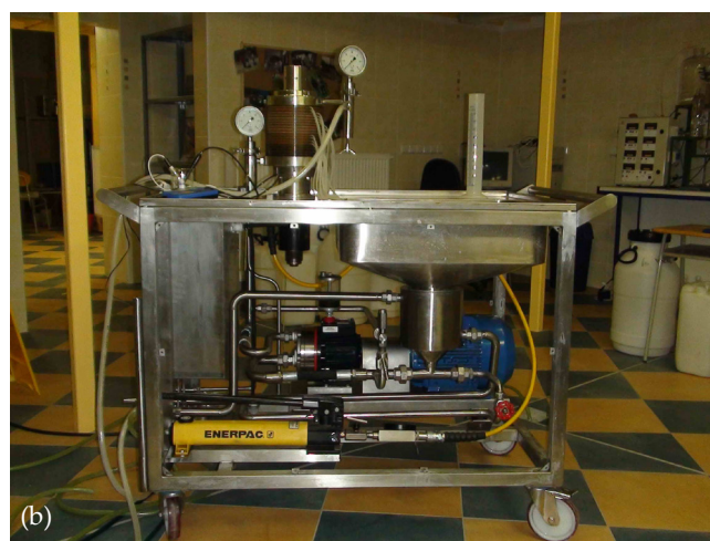
Fig. 2. Reverse osmosis pilot scale unit LAB-M20: (a) schematic representation, (b) total view.
