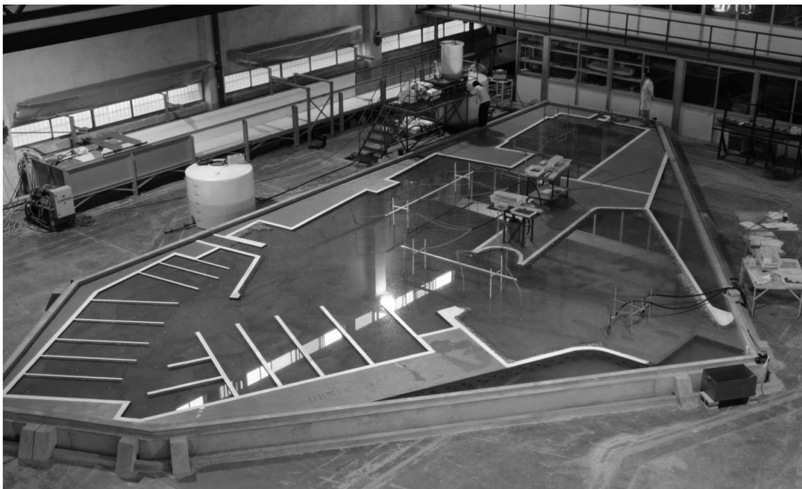
Fig. 1. Physical model of the harbour of Denia at 1:65 scale.
