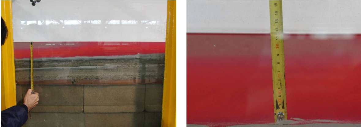
Fig. 10. Because of the rhodamine stained, it can be estimated the plunged area (left) or the thickness of the hyperdense layer (right).
