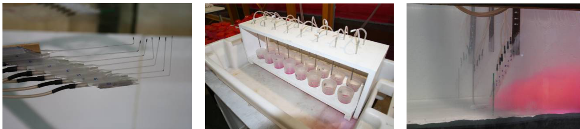
Fig. 16. Pasteur pipettes and peristaltic pump taking out liquid during a test.
