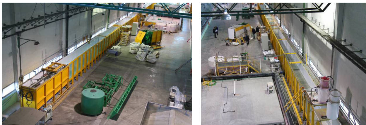
Fig. 7. Wave flume in the Centre for Harbours and Coastal Studies of CEDEX.
