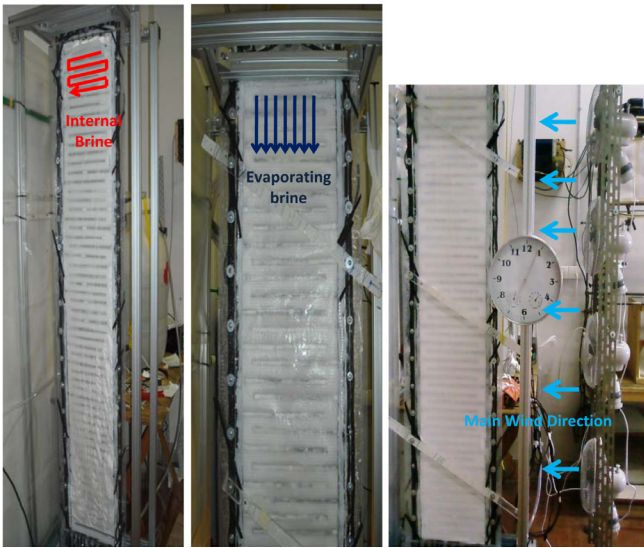
Fig. 5. Overviews of the laboratory pilot unit with indications of the flow directions for the two streams and the wind generated by four fans.
