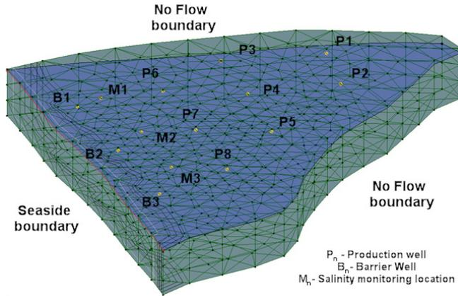
Fig. 1. Three dimensional view of the well field discretized into finite elements.
