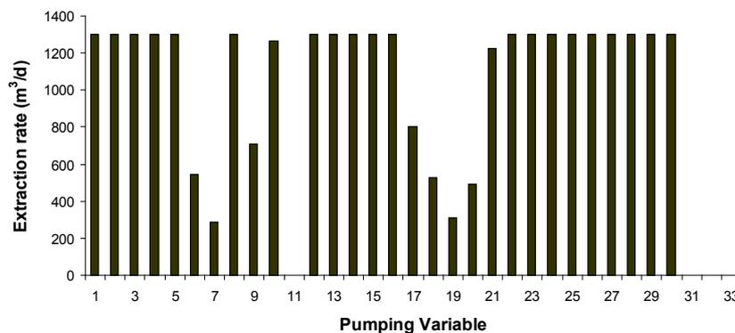
Fig. 5. Optimal pumping rates corresponding to total barrier well pumping of 4121 m<sup>3</sup>/d.
