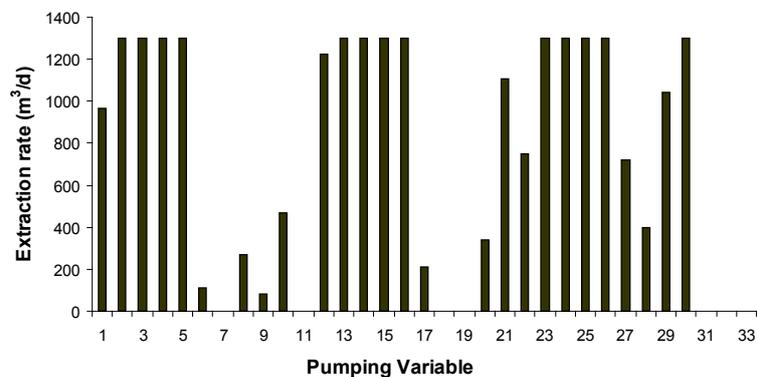
Fig. 3. Optimal pumping rates corresponding to total barrier well pumping of 2037 m<sup>3</sup>/d.
