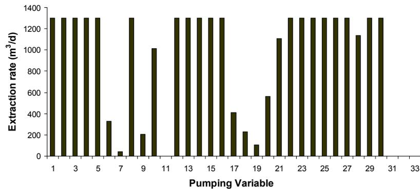
Fig. 4. Optimal pumping rates corresponding to total barrier well pumping of 3094 m<sup>3</sup>/d.
