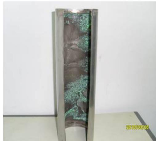
Fig. 3. The photo of cathode after reaction. Conditions:  $[H_3BO_3] = 0.5$  g/L,  $V = 1.4$  L, current density =  $2.0$  A/dm<sup>2</sup> (current  $10.6$  A), pH =  $2.2 \pm 0.3$ .
