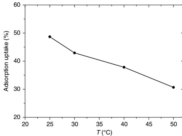
Fig. 4. Effect of temperature on the adsorption uptake of copper (II) from aqueous solution onto zeolite NaY.  $[Cu^{2+}] = 100$  mg/l, pH  $(Cu^{2+}) = 5$  and S/L = 2.5.
