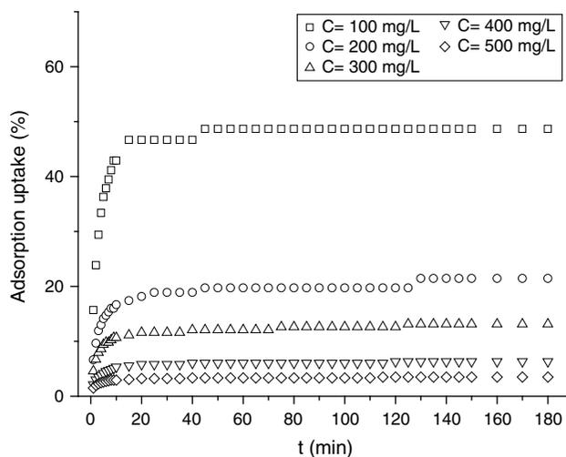
Fig. 2. Adsorption uptake of  $\text{Cu}^{2+}$  ions onto NaY zeolite as versus the contact time by varying the metal concentration from 100 to 500 mg/l.  $T = 298 \text{ K}$ ,  $\text{pH} = 5$  and  $S/L = 2.5$ .
