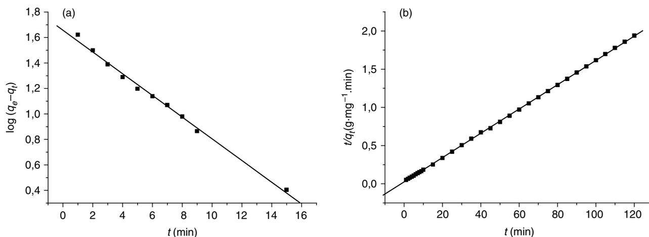
Fig. 6. Pseudo-first order (a) and Pseudo-second order (b) kinetic plots for the sorption of copper (II) ions from aqueous solutions on zeolite NaY.  $T = 298$  K,  $[\text{Cu}^{2+}] = 100$  mg/l, pH = 5 and S/L = 2.5.
