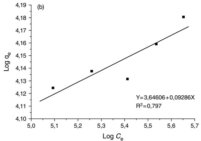
Fig. 5. Langmuir (a) and Freundlich (b) isotherms for adsorption of copper (II) on zeolite NaY.  $T = 298$  K,  $[Cu^{2+}] = 100$  mg/l, S/L = 2.5 and pH = 5.
