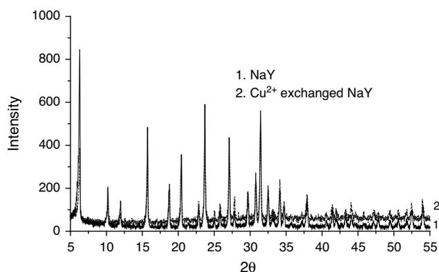
Fig. 1. XRD patterns of (1) NaY and (2)  $\text{Cu}^{2+}$  exchanged NaY.
