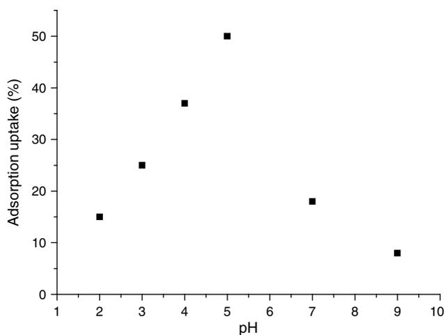
Fig. 3. Effect of pH on the adsorption uptake of copper (II) from aqueous solution onto NaY zeolite.  $T = 298 \text{ K}$ ,  $[\text{Cu}^{2+}] = 100 \text{ mg/l}$  and  $S/L = 2.5$ .
