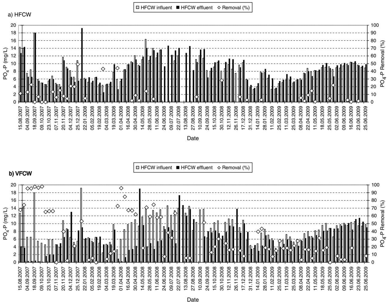
Fig. 2. Influent and effluent  $\text{PO}_4$ -P concentrations and removal efficiencies in a) HFCW and b) VFCW.
