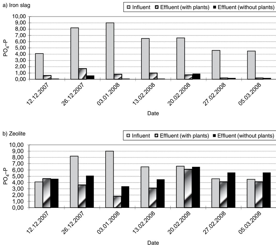
Fig. 5. Influent and effluent  $\text{PO}_4\text{-P}$  concentrations in 1 m<sup>2</sup> wetlands (P-HFCW) filled with a) iron slag and b) zeolite.
