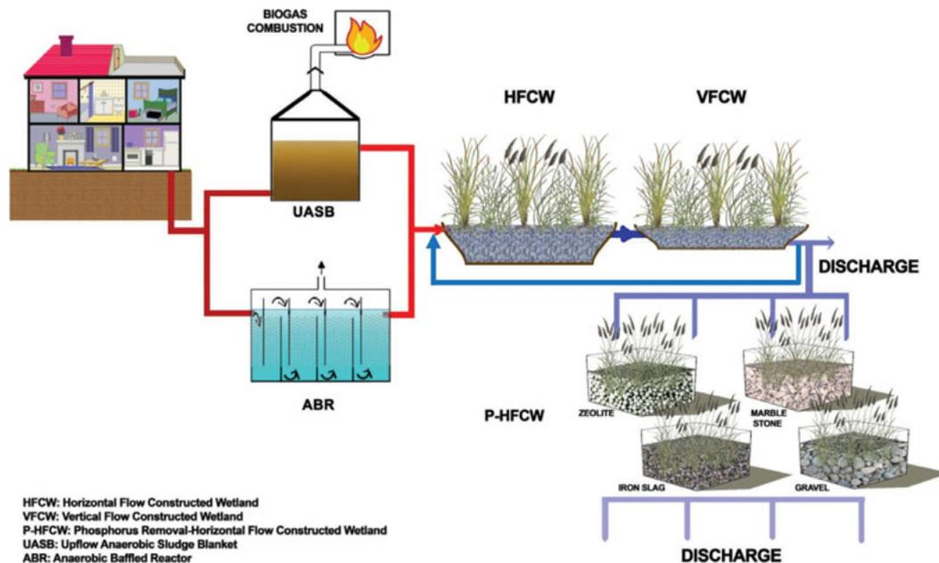
Fig. 1. Flow diagram of the hybrid constructed wetland system with anaerobic pretreatment.
