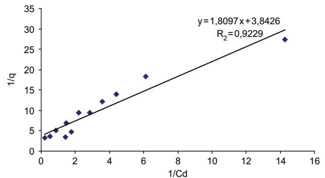
Fig. 3. Adsorption isotherm for PO<sub>4</sub>-P obtained for iron slag.
