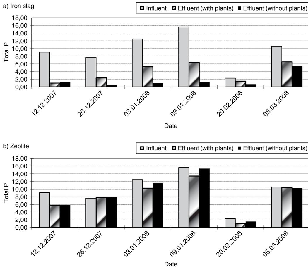
Fig. 4. Influent and effluent total P concentrations in 1 m<sup>2</sup> wetlands (P-HFCW) filled with a) iron slag and b) zeolite.
