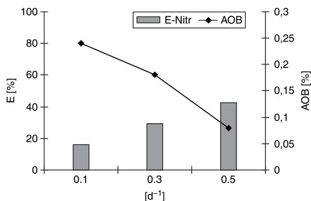
Fig. 3. AOB percentage in activated sludge in relation to volumetric exchange rate.
