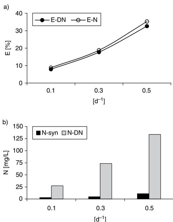
Fig. 4. Efficiency of denitrification (E-DN) and nitrogen removal (E-N) (a), the amount of nitrogen removed by denitrification (N-DN) and for biomass synthesis (N-syn) (b) at different volumetric exchange rate.
