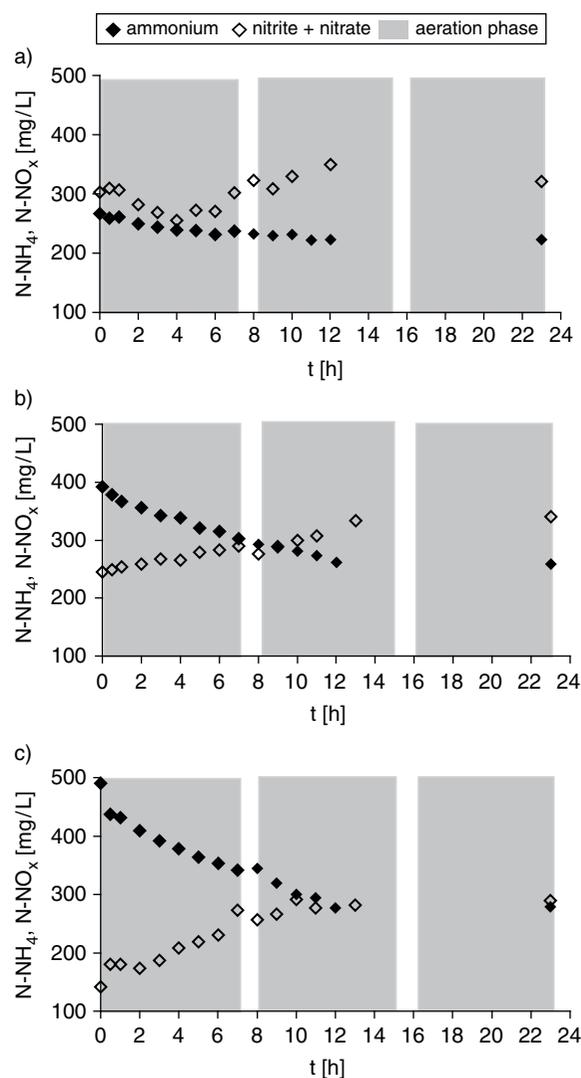
Fig. 1. Ammonium removal and nitrite and nitrate formation in the SBR cycle; a) series 1, b) series 2, c) series 3.
