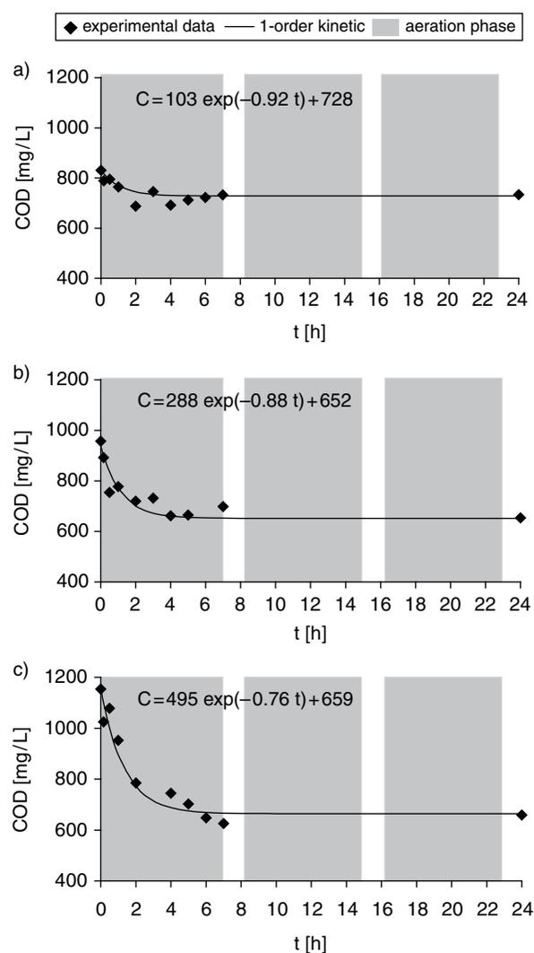
Fig. 2. COD removal during the SBR cycle; a) series 1, b) series 2, c) series 3.
