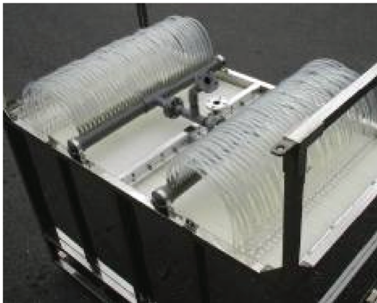
Fig. 3. Non-woven membrane module used in this case study.
