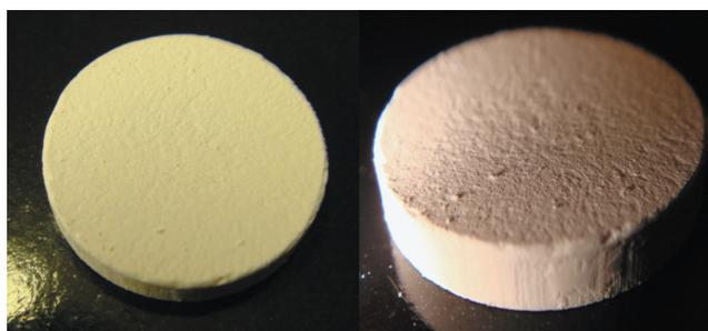
Fig. 5.  $\alpha$ -alumina substrate before (green compact) and after sintering.
