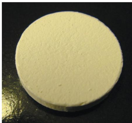
Fig. 3. Green  $\alpha$ -alumina compact pressed at 620 MPa.
