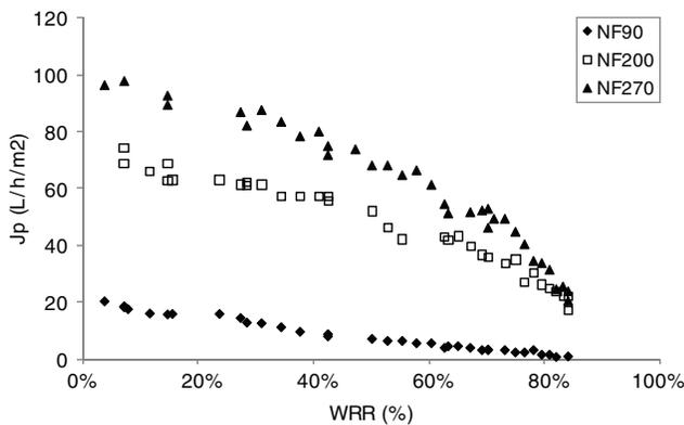
Fig. 6. Variation of NF90 ( $\blacklozenge$ ), NF200 ( $\square$ ) and NF270 ( $\blacktriangle$ ) permeate fluxes as a function of water recovery rate (WRR) for the raw sado river water. Transmembrane pressure: 30 bar and Temperature: 25°C (sample collected in June).
