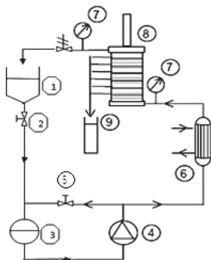
Fig. 2. Nanofiltration DSS Lab-unit M20 set-up.
