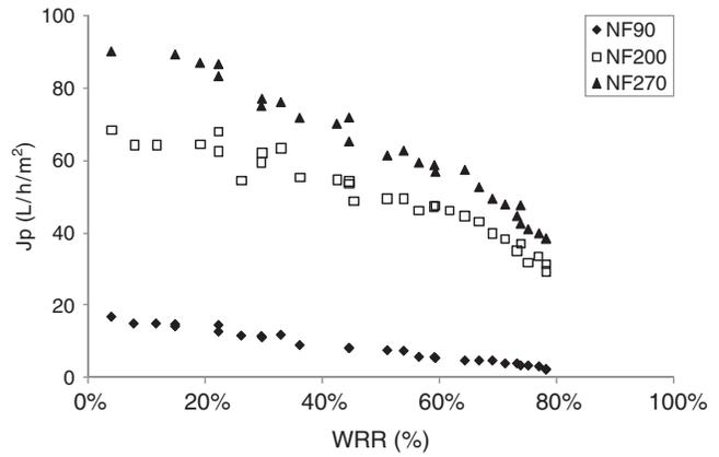
Fig. 7. Variation of NF90 ( $\blacklozenge$ ), NF200 ( $\square$ ) and NF270 ( $\blacktriangle$ ) permeate fluxes as a function of water recovery rate (WRR) for the EDs Inoculated Sado river water. Transmembrane pressure: 30 bar and Temperature: 25°C (sample collected in June).
