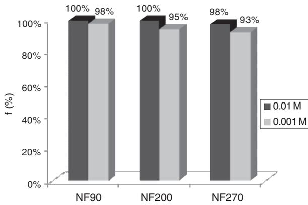
Fig. 5. Variation of humic acid average apparent rejection coefficients ( $f$ ) with ionic strength ( $10^{-2}$  M and  $10^{-3}$  M) for NF90, NF200 and NF270 membranes. Feed circulation flow-rate: 0.6 l/min, operating pressure: 10–35 bar.
