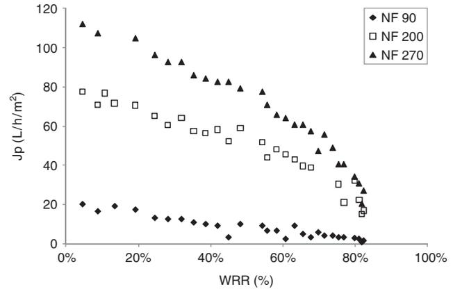
Fig. 8. Variation of NF90 ( $\blacklozenge$ ), NF200 ( $\square$ ) and NF270 ( $\blacktriangle$ ) permeate fluxes as a function of water recovery rate (WRR) for the raw sado river water. Transmembrane pressure: 30 bar and Temperature: 25°C (sample collected in October).
