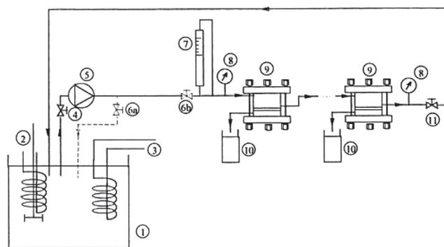
Fig. 1. Nanofiltration flat-cell unit set-up.
