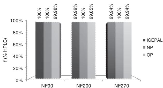
Fig. 3. Variation of rejection coefficients ( $f$ ) to IGEPAL, NP and OP for membranes NF90, NF200 and NF270. Feed circulation flowrate: 0.6 l/min, operating pressure: 30 bar.
