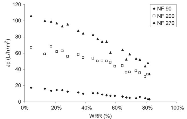
Fig. 9. Variation of NF90 ( $\blacklozenge$ ), NF200 ( $\square$ ) and NF270 ( $\blacktriangle$ ) permeate fluxes as a function of water recovery rate (WRR) for the Inoculated sado river water. Transmembrane pressure: 30 bar and Temperature: 25°C (sample collected in October).
