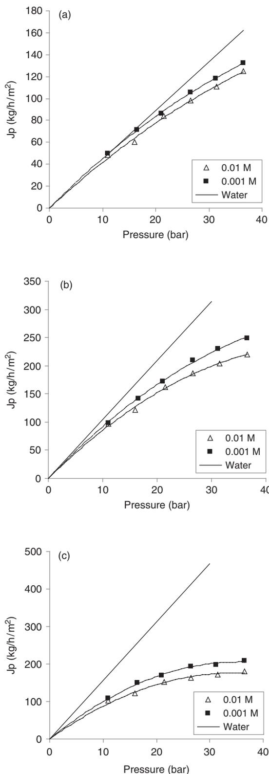
Fig. 4. Variation of permeation fluxes with pressure for the membranes NF90 (a), NF200 (b) and NF270 (c). Model solution of humic acid (10 mg/l) and ionic strengths of  $10^{-2}$  M and  $10^{-3}$  M. Feed circulation flowrate: 0.6 l/min, operating pressure: 10–35 bar.
