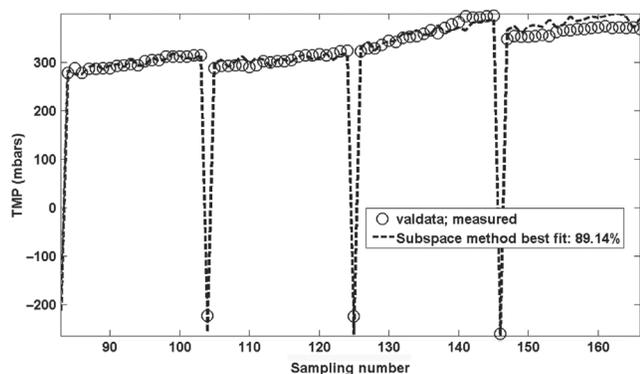
Fig. 7. Pilot membrane filtration unit - best model fit for 8 flux steps (4 for validation) for Subspace method.
