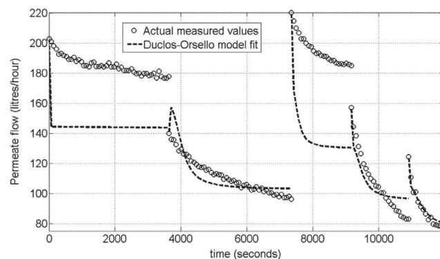
Fig. 2. Pilot MBR plant - best model fit for 5 flux steps.
