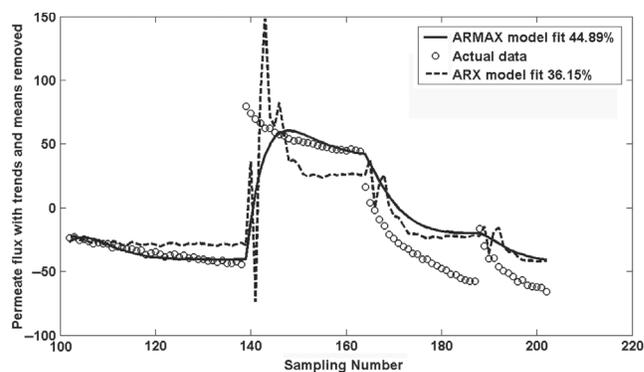
Fig. 6. Pilot MBR plant - best model fit for 7 flux steps (4 for validation) for ARX and ARMAX formulations.
