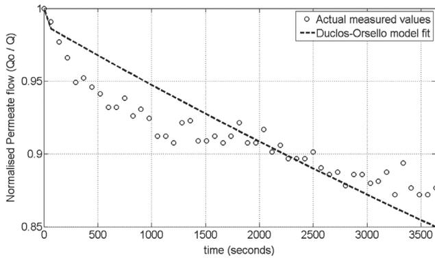
Fig. 3. Pilot MBR plant - best model fit for single flux step.
