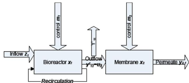
Fig. 1. Part of a “model conceptualisation procedure” used to develop rational relationships between IO variables for an approximate decomposed MBR model (Source: Paul 2010).
