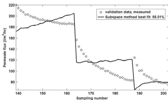
Fig. 5. Pilot MBR plant - best model fit for 7 flux steps (3 for validation) for Subspace method.
