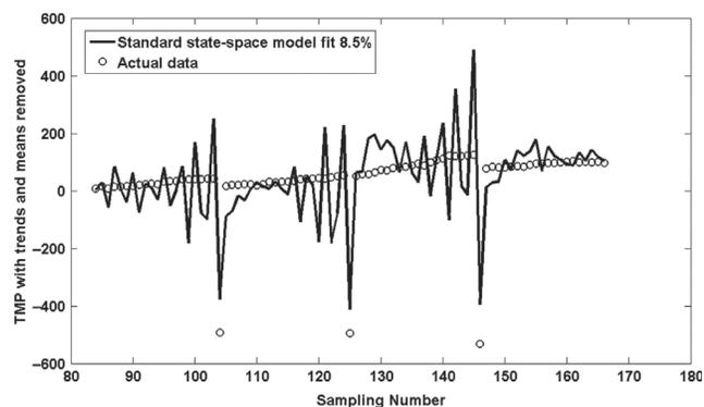
Fig. 8. Pilot membrane filtration unit - best model fit for 8 flux steps (4 for validation) for standard state-space formulation.
