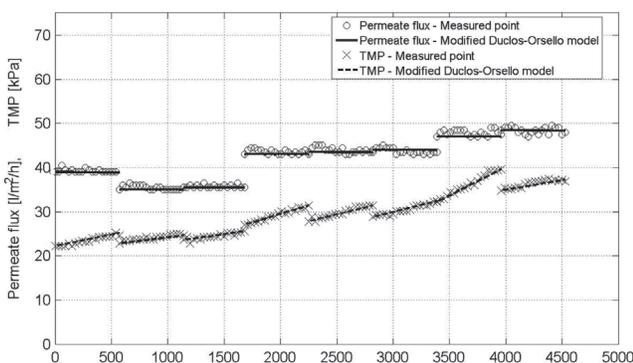
Fig. 4. Pilot membrane filtration unit - best model fit for 8 flux steps.
