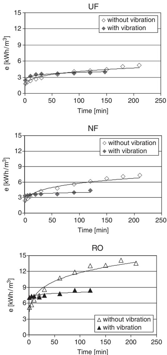
Fig. 9. Specific energy demand per m<sup>3</sup> permeate during concentration experiments.
