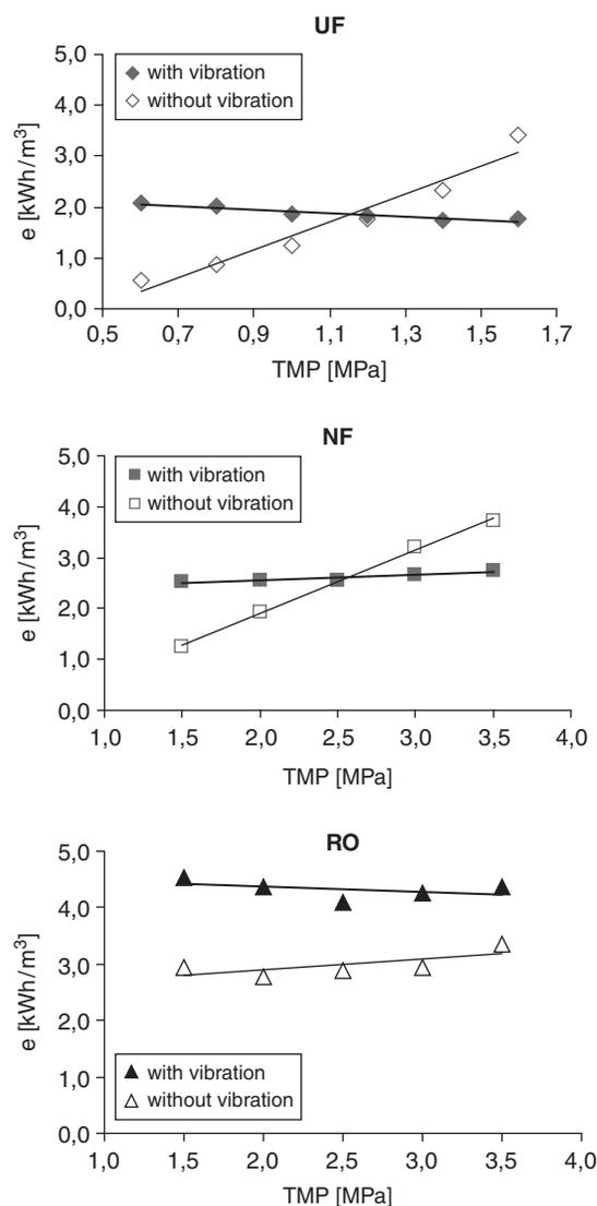
Fig. 8. Specific energy demand per  $\text{m}^3$  permeate with and without vibration during UF, NF and RO.
