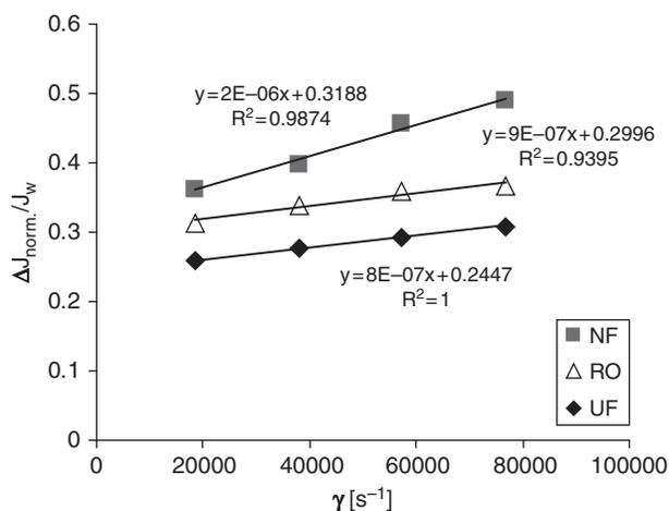
Fig. 5. Increment in the flux differences in relation to mean shear rate during vibration UF, NF and RO.
