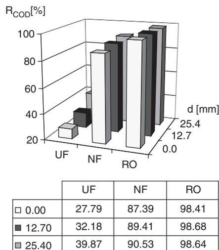
Fig. 6. The effect of vibration amplitude on COD rejection during UF, NF and RO.
