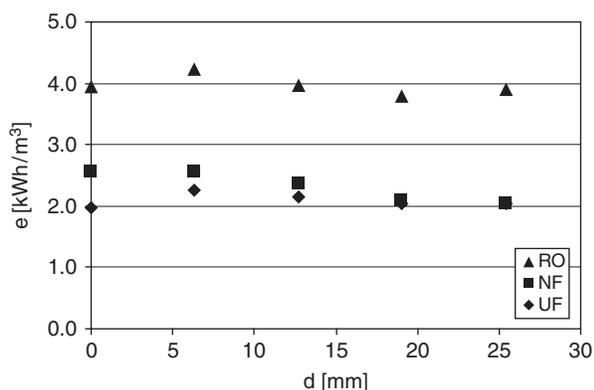
Fig. 7. The specific energy demand of the feed pump and vibratory module in the function of vibration amplitude.
