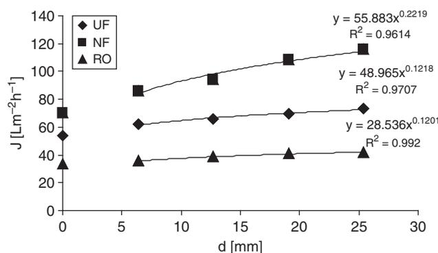
Fig. 4. Flux in relation to vibration amplitude during UF, NF and RO.
