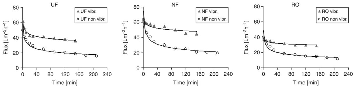
Fig. 1. Permeate flux vs. time during UF, NF and RO without and with membrane vibration.
