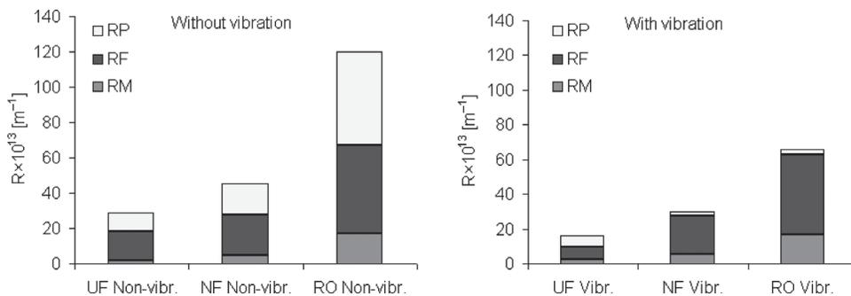
Fig. 3. The content of total membrane resistances without and using vibration during UF, NF and RO.
